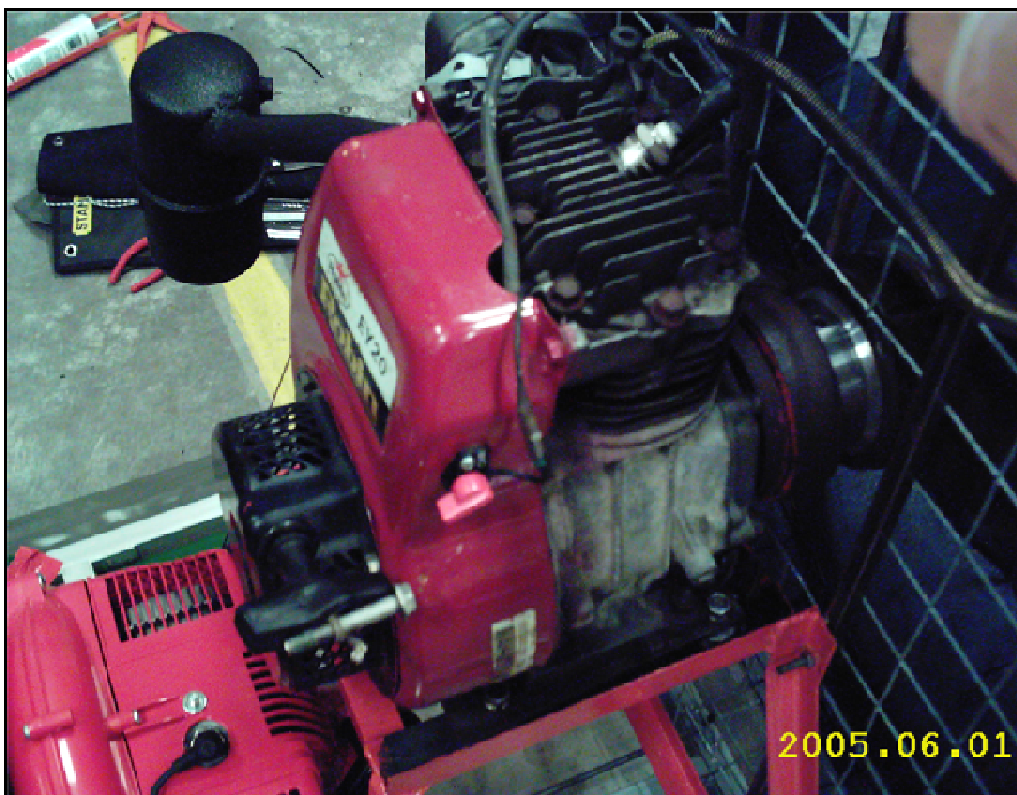
Figure 1. Lifting and thrusting engines; (a) air blower (lifting) and (b) thrust engine (thrusting).
