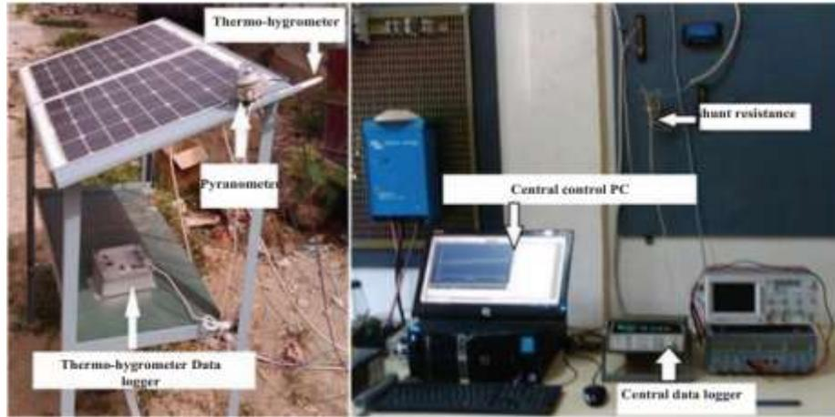
Figure 1. Photovoltaic platform of measurements.
