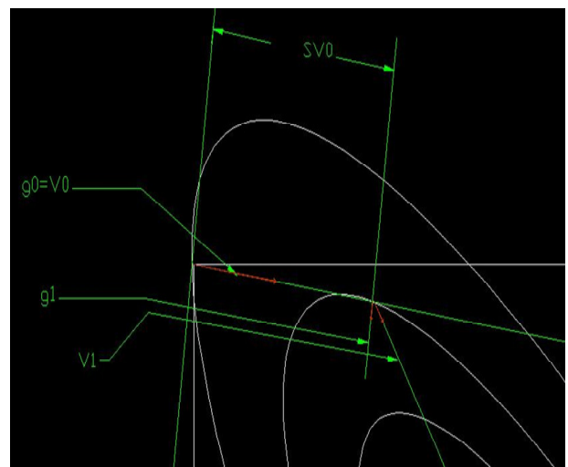
Figure 3. Geometric representation of potential dynamic work for a function of two variables.
