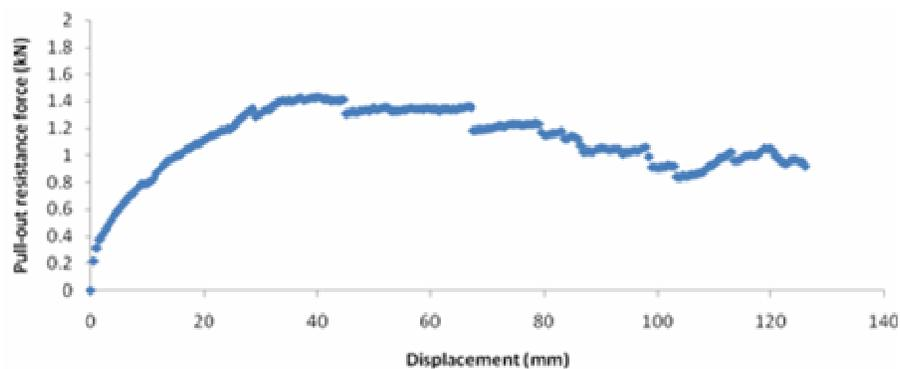
**Figure 7.** Average pull-out resistance force-displacement curve for a pull-out test on five replicates *M. malabathricum*.
