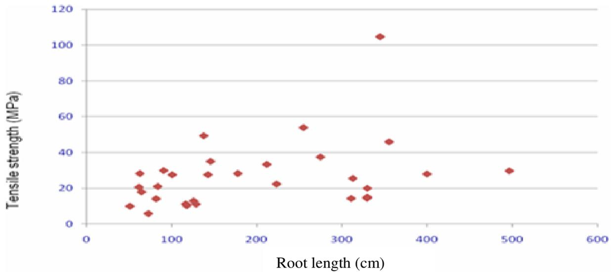
Figure 17. There is no well correlated relationship observed between tensile strength and root length.
