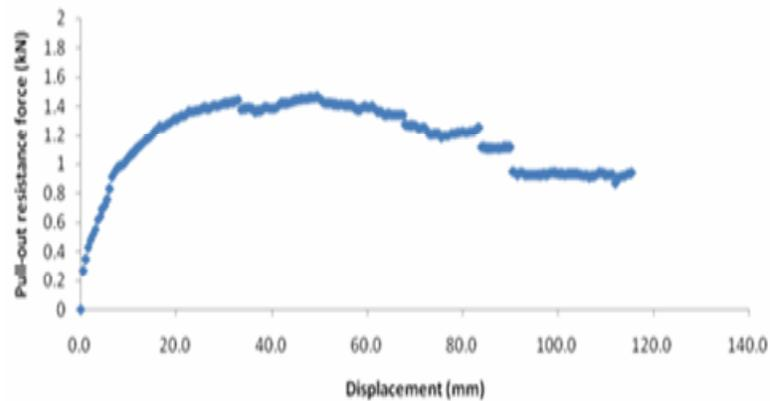
**Figure 5.** Average pull-out resistance force-displacement curve for a pull-out test on five replicates *A. mangium*.
