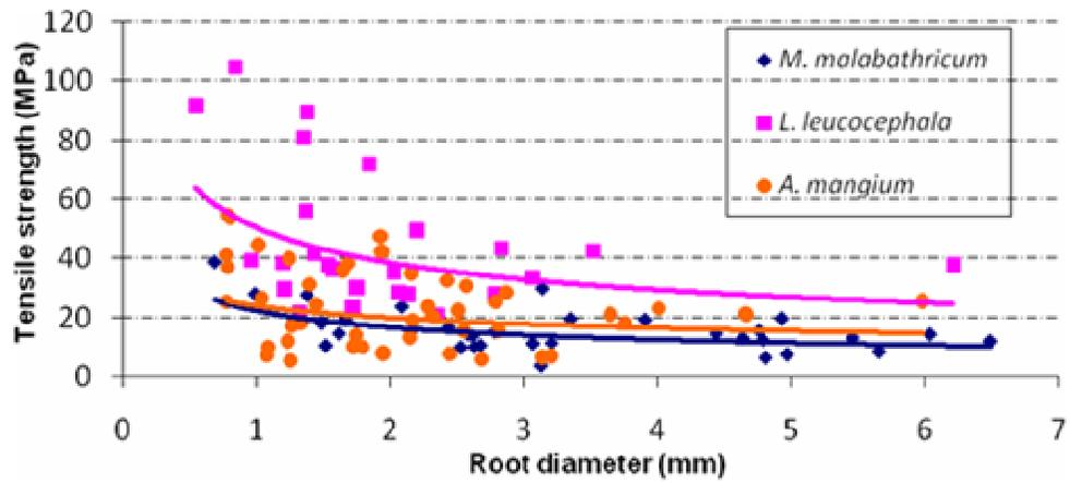
Figure 16. Relationship between tensile strength and root diameter.
