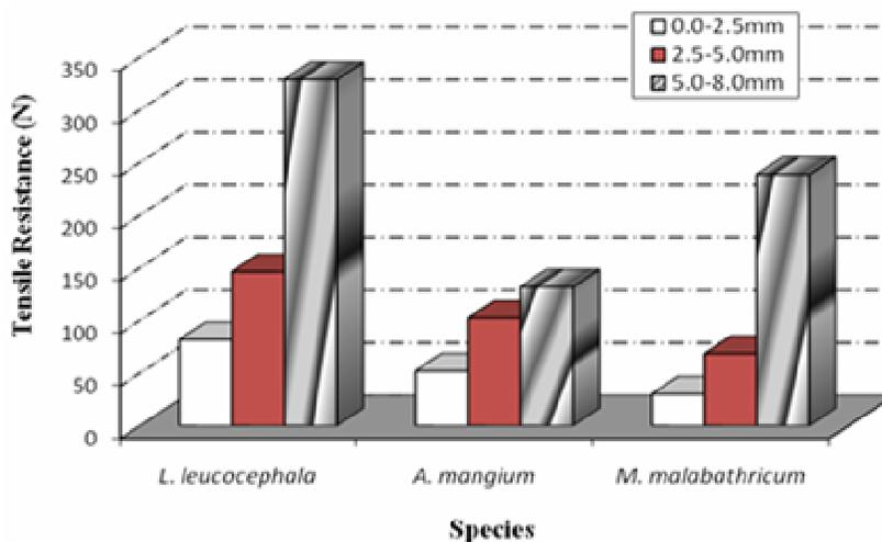
Figure 13. Tensile resistance at certain root diameter.
