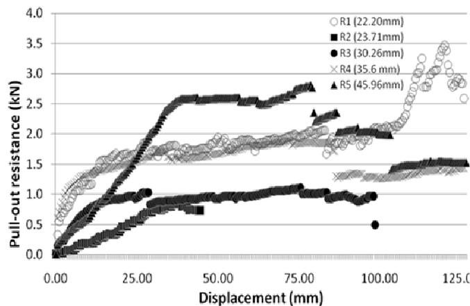
**Figure 4.** Plots of pull-out resistance versus displacement for *M. malabathricum*.
