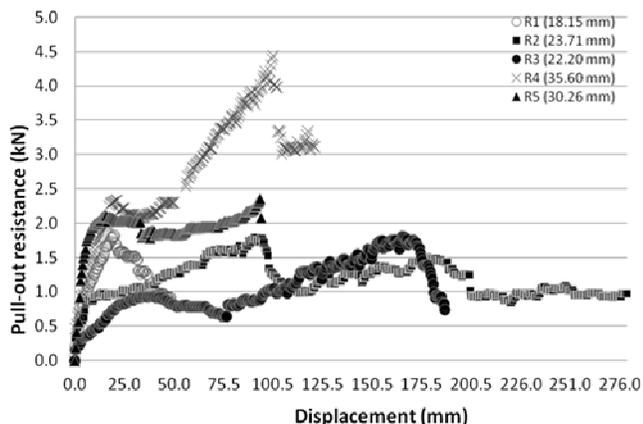
**Figure 3.** Plots of pull-out resistance versus vertical displacement for *L. leucocephala*.
