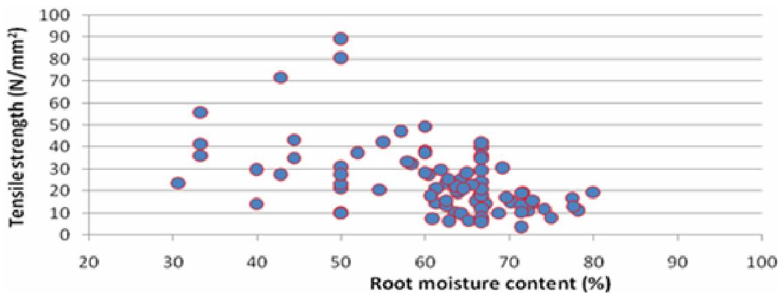
Figure 18. Relationship between tensile strength and root moisture content.
