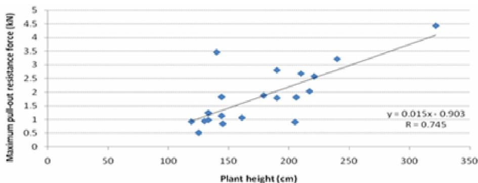
**Figure 9.** The relationship between the maximum pull-out resistance force and the plant height for all species.
