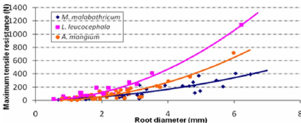
Figure 15. Relationship between maximum tensile resistance and root diameter.
