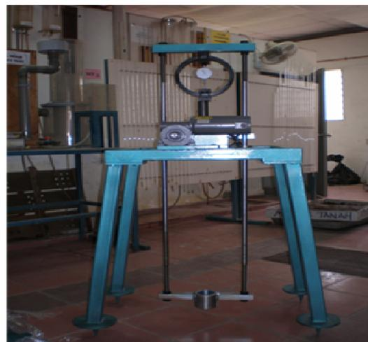
**Figure 1.** Pull-out test apparatus was fabricated for 0-60 mm of stem diameter.
