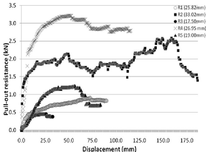
**Figure 2.** Plots of pull-out resistance versus displacement for *A. mangium*.
