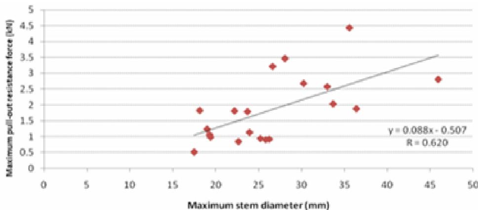
**Figure 8.** The relationship between the maximum pull-out resistance and the maximum stem diameter for all species.
