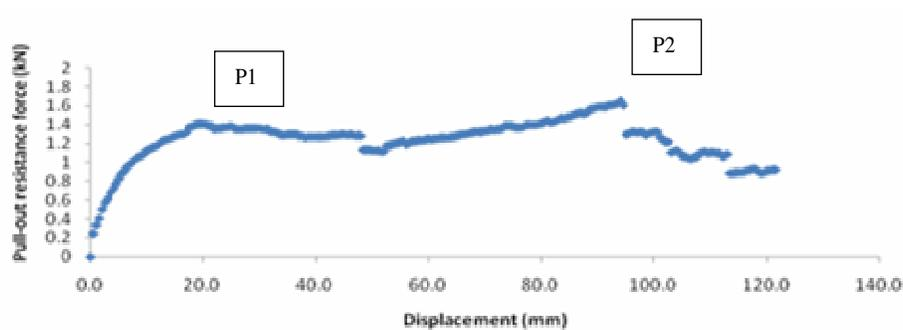
**Figure 6.** Average pull-out resistance force-displacement curve for a pull-out test on five replicates *L. leucocephala*. P1 and P2 contributed by lateral and tap roots, respectively.
