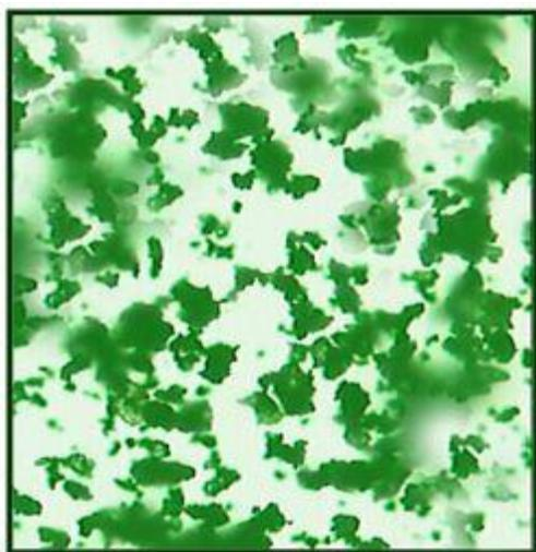
**Figure 11.** Optical polarized micrographs of random copolyester
