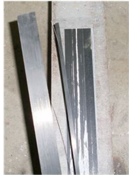
Figure 7. End delaminating (EDL).
