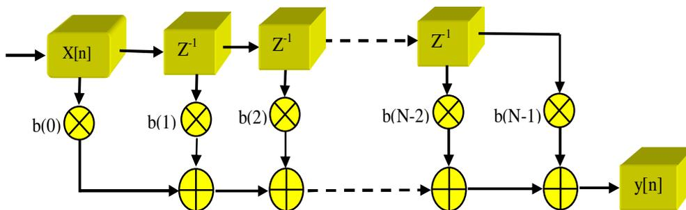
Figure 3. General structure of FIR filter (Proakis and Manolakis, 2006).
