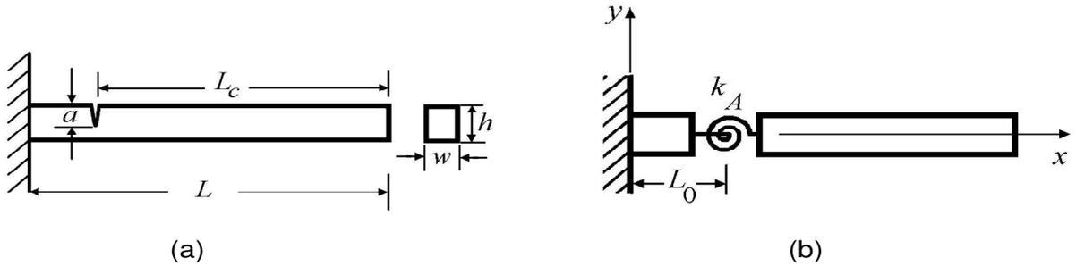
**Figure 1.** (a) Cantilever beam with a breathing crack; (b) a nonlinear stiffness model for the breathing crack on a cantilever beam.
