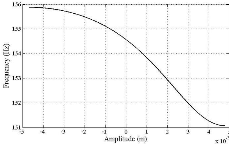
**Figure 4.** The range of the natural frequency changes of the cracked beam with the crack parameters of  $\alpha = 0.36$  and  $\beta = 0.81$  against the vibration amplitude.
