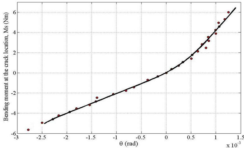
**Figure 2.** The variation of bending moment against the local slope difference at the crack location for a steel cracked beam with a cross-sectional area of  $3.9 \times 6.4 \text{ mm}^2$  and a crack depth ratio of  $\alpha = 0.36$  obtained through the experimental tests (●) and the curve fitted to the experimental test points (—).
