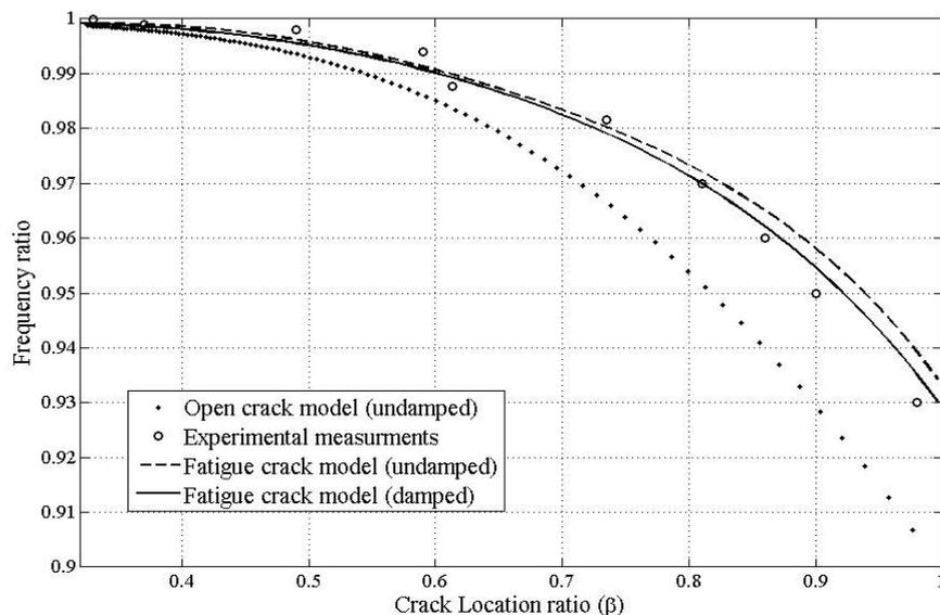
**Figure 8.** Variation of the fundamental frequency ratio of the cracked cantilever beam against the crack location ratio for the crack depth ratio of  $\alpha = 0.36$  obtained from the proposed method based on the fatigue crack model by taking into account the effects of the system damping (—), fatigue crack model without taking into account the effects of the system damping (---), undamped open crack model (· · ·) and the experimental results (o).
