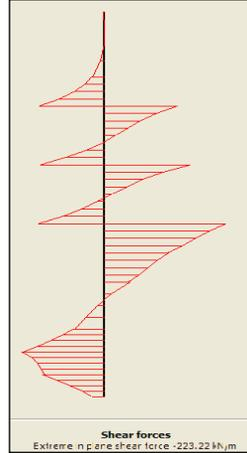
Figure 32. Shear Force ( $\phi=13^\circ$ ,  $c=32 \text{ kN/m}^2$  and  $H_w=20 \text{ m}$ )
