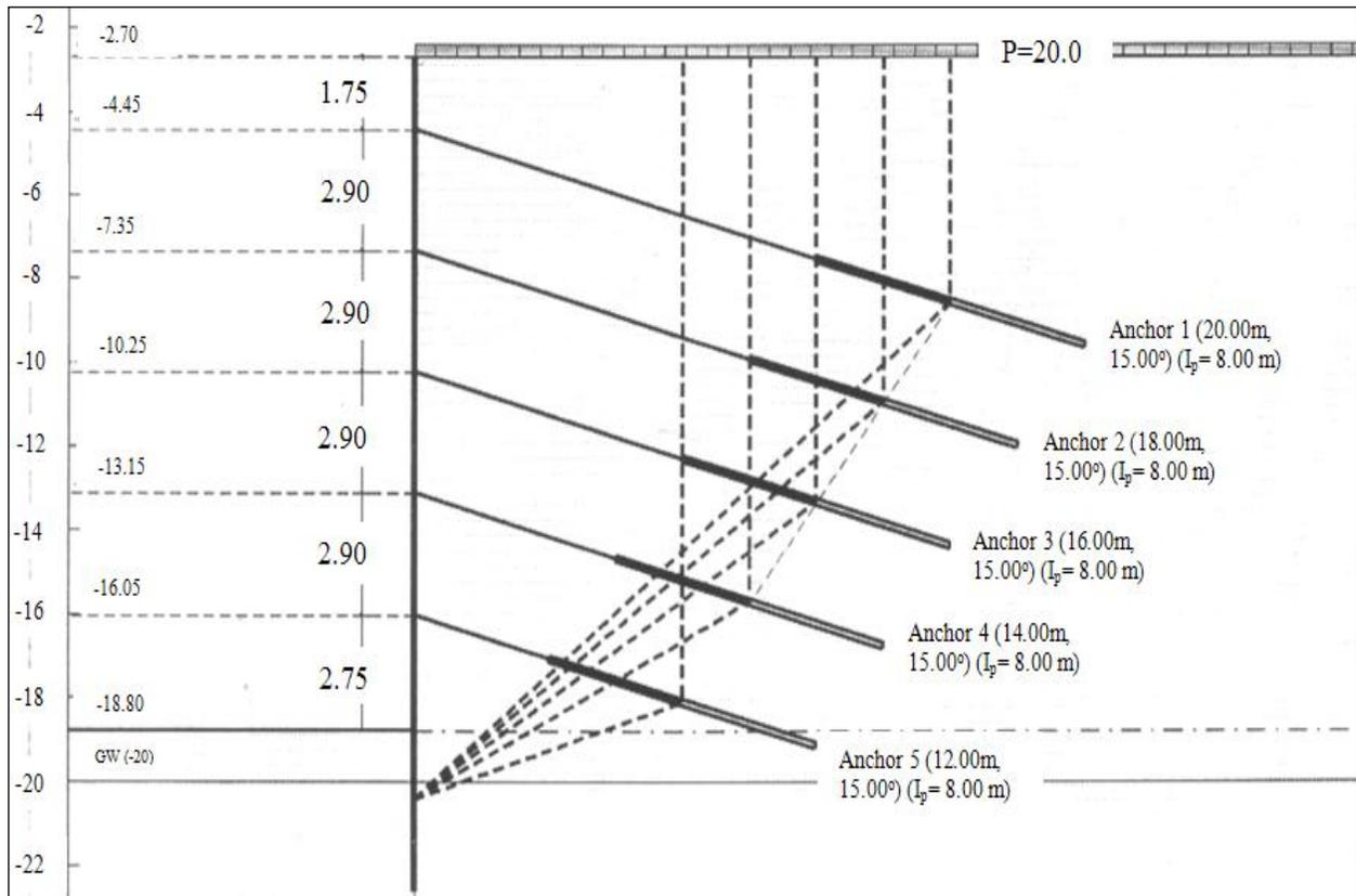
Figure 4. Road Elevation of the Excavation Site A-A section
