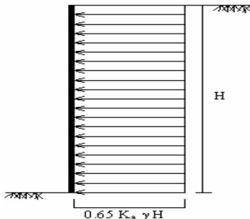
**Figure 13.** Lateral Soil Pressure Distributions Suggested by Terzaghi-Peck for the Noncohesive Soils (Terzaghi-Peck, 1967)
