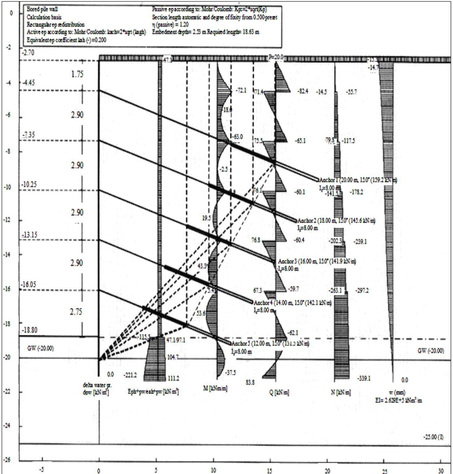
Figure 6. Moment, Shear, Normal Load, and Bending Rigidity Distributions of Collapsed Retaining System
