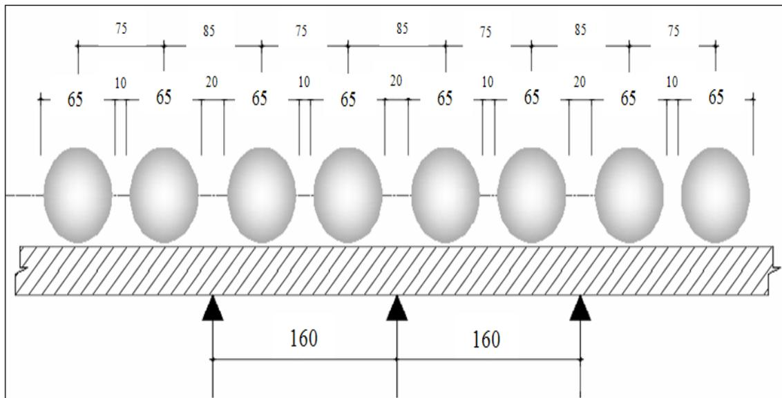
Figure 5. Pile and Anchor Modulation Plan
