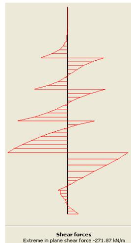
Figure 38. Shear Force ( $\phi=13^\circ$ ,  $c=32$  kN/m<sup>2</sup> and  $H_w=11$  m) (Hardening Soil Method)
