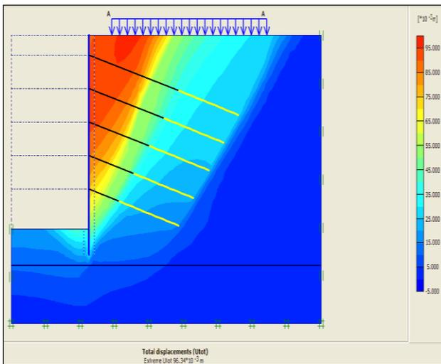
Figure 16. After The Analysis of Total Displacement
