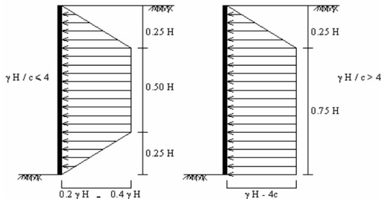
**Figure 14.** Lateral Soil Pressure Distributions Suggested by Peck for the Cohesive Soils (Peck, 1969)
