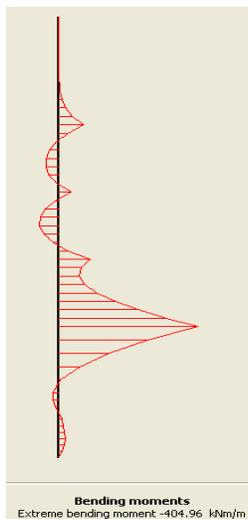
Figure 37. Bending Moment ( $\phi=13^\circ$ ,  $c=32$  kN/m<sup>2</sup> and  $H_w=11$  m) (Hardening Soil Method)
