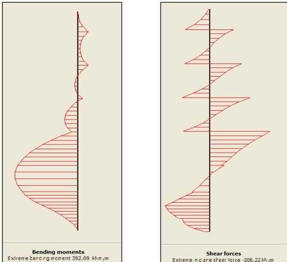
Figure 25. Bending Moment ( $\phi=13^\circ$ ,  $c=32 \text{ kN/m}^2$  and  $H_w=11 \text{ m}$ ) (Mohr – Coulomb Method)
