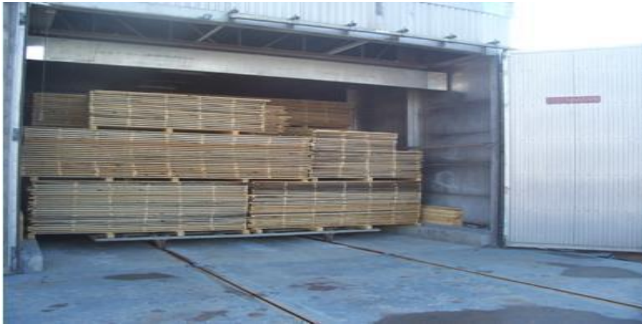
Figure 3. The kiln and sample boards.
