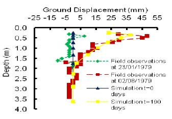
**Figure 4.** Simulated and site ground displacements profiles after 190 days at radial distance of 1.4 m from lime tree.
