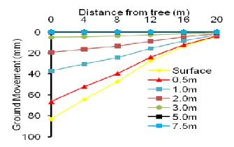
**Figure 2.** Variation of ground movement with depth near the tree for the current research.
