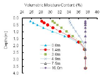
**Figure 7.** Variations of volumetric moisture content with depth at various lateral distance from lime tree after 270 days.
