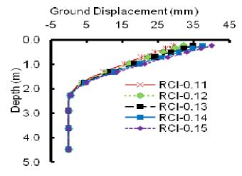
**Figure 12.** Variation of ground settlement with depth at various soils re-compression index at 3.0 m away from lime tree after 190 days.
