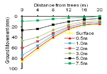
**Figure 3.** Variation of ground movement with depth near the tree after Fredlund and Hung (2001).
