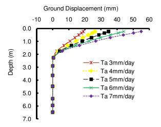
**Figure 9.** Variation of ground settlement with depth at various potential transpiration rates at 3.0m away from lime tree after 190 days.
