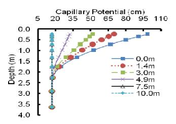
**Figure 6.** Variations of capillary potential with depth at various lateral distance from lime tree after 190 days.
