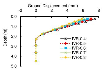
**Figure 11.** Variation of ground settlement with depth at various initial void ratios at 1.4m from lime tree after 30 days.
