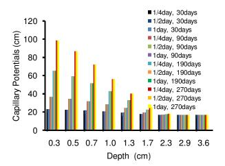
**Figure 8.** Variations of time step size with capillary potential and depth at 1.4 m from the lime tree after 30, 90, 190 and 270 days.
