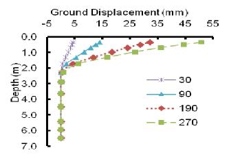
**Figure 5.** Variations of ground settlement with depth at various elapse time at 3.0 m away from the lime tree in days.
