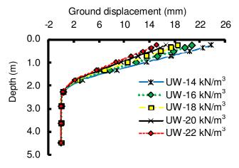
**Figure 10.** Variation of ground settlement with depth at various unit weights of the soil at 4.9 m away from lime tree after 190 days.
