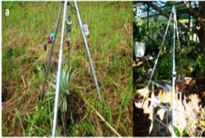
Figure 2. Tensile force measurement of plant roots on experimental prototype slope (a) and pots (b).
