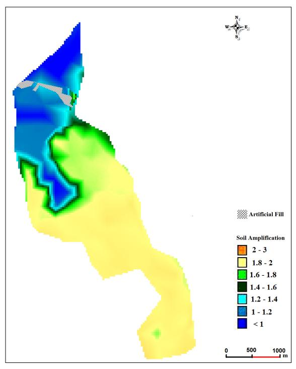
Figure 10. Soil amplification values in the study area according to Midorikawa (1987) relation.
