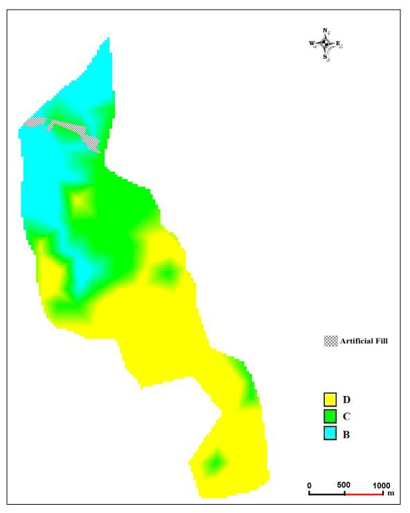
Figure 5. Soil classification according to NEHRP (2001, BSSC).
