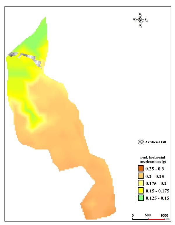
**Figure 7.** Variation of average peak horizontal accelerations estimated attenuation relationships (Boore et al., 1997; Gülkan and Kalkan, 2002).
