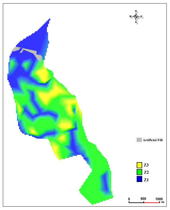
Figure 4. Soil classification according to Turkish earthquake code (TEC, 2007).
