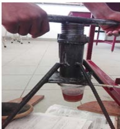
Figure 2. Prototype hydraulic press (a-closing diameter 5.7cm, b –internal diameter 6.1 cm, c-external diameter 6.8 cm, d-depth 17.37 cm, and e-closing height 19.0 cm).
