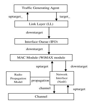
Figure 2. NS2 architecture and WiMAX module.
