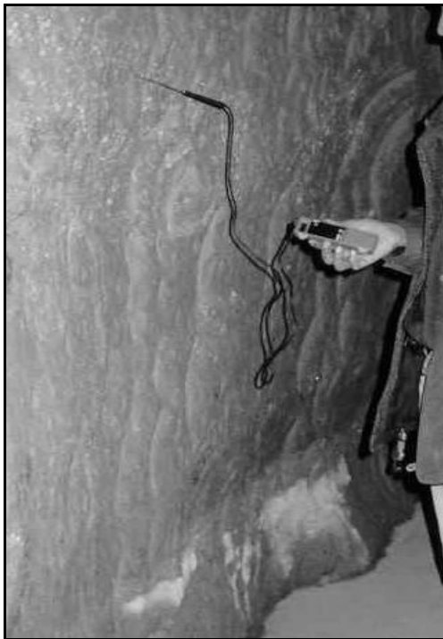
Figure 9. Heat conductivity measurements in the wall of the cavern.
