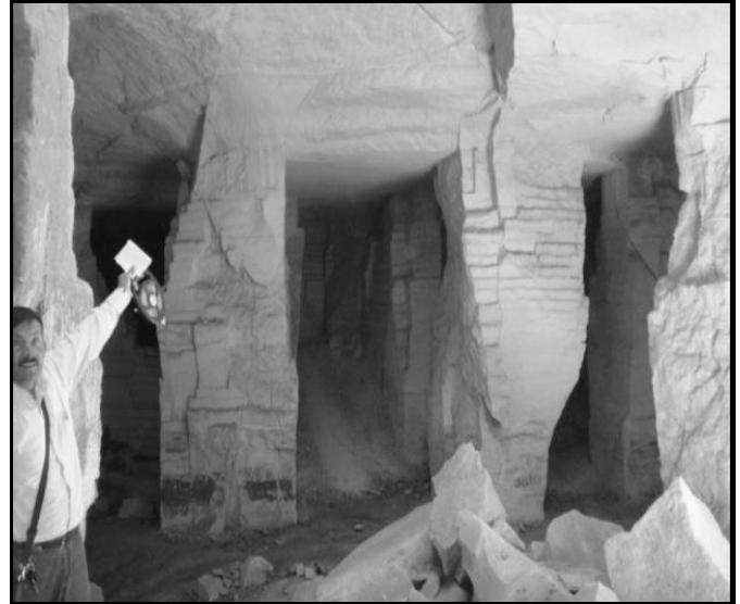
Figure 7. Pillars of a cavern which used for quarry
