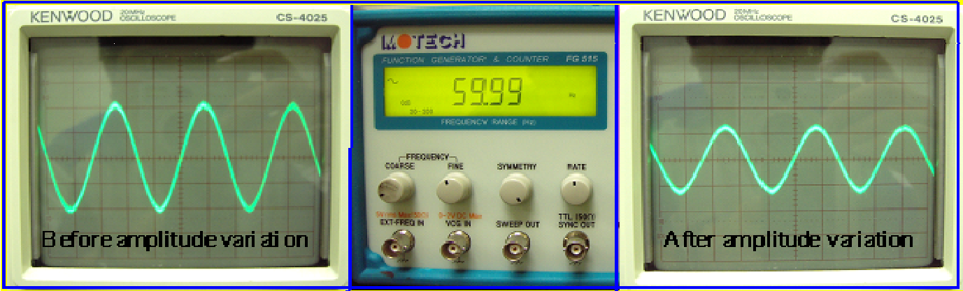
Figure 2. The wave form of function generator by oscilloscope display.
