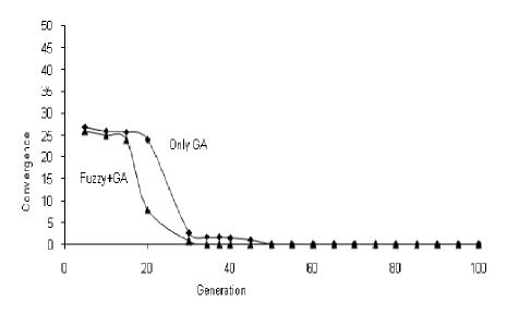
Figure 4. Convergences versus generations for 3 DOF robotic system.
