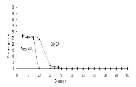
Figure 5. Convergence versus generation for 4 DOF robotic system.
