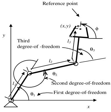
Figure 1. Three degree-of -freedom manipulator.
