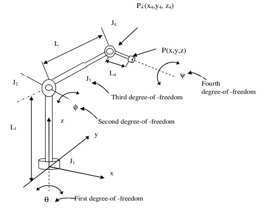
Figure 2. Four degree-of -freedom manipulator.
