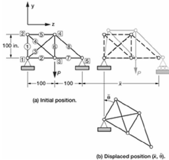
Figure 2. Eight-bar truss.
