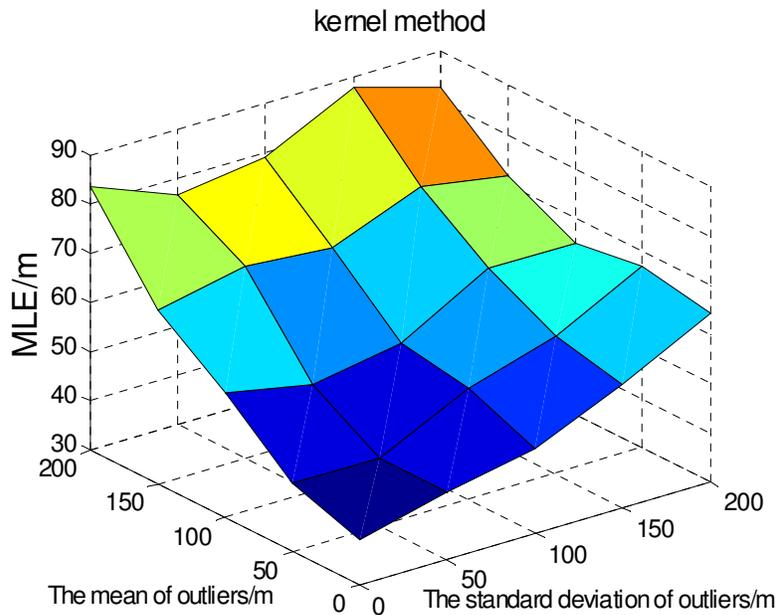
**Figure 4.** Mean location error versus the standard deviation and mean of outliers in kernel method.
