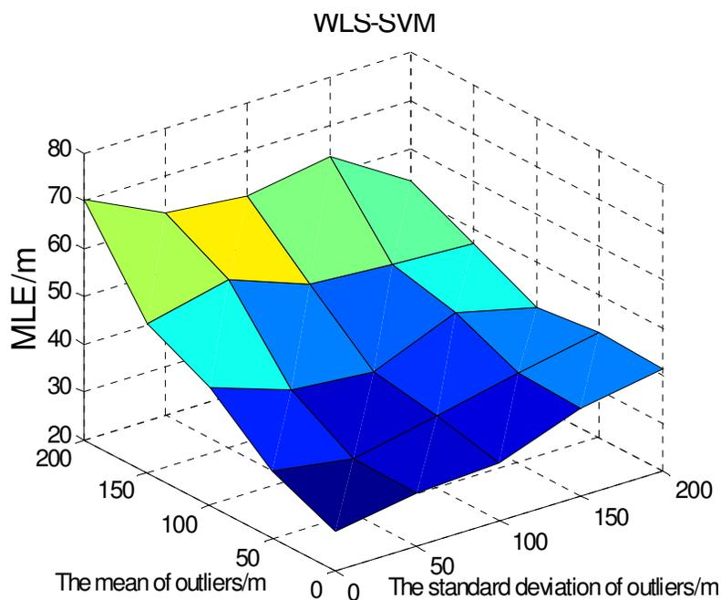
**Figure 6.** Mean location error versus the standard deviation and mean of outliers in WLS-SVM method.
