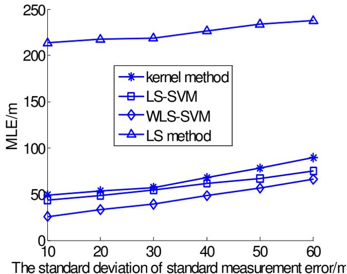
**Figure 7.** Performance comparison with difference standard deviation of standard measurement error.
