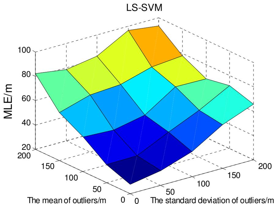
**Figure 5.** Mean location error versus the standard deviation and mean of outliers in LS-SVM method.
