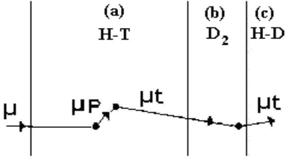
**Figure 1.** Muons of momentum  $26.25 \text{ MeV}/c$  are injected into the multilayered solid target  $H-T/D_2/H-D$ . The  $\mu t$  emission is based on the RT effect: (a) the  $H/T$  layer adopted with a small amount tritium impurity for production of fast muonic atoms, (b) deuterium moderator, (c) a fusion layer of  $H-D$ . The most of released muons by fusion stay in the fusion layer.
