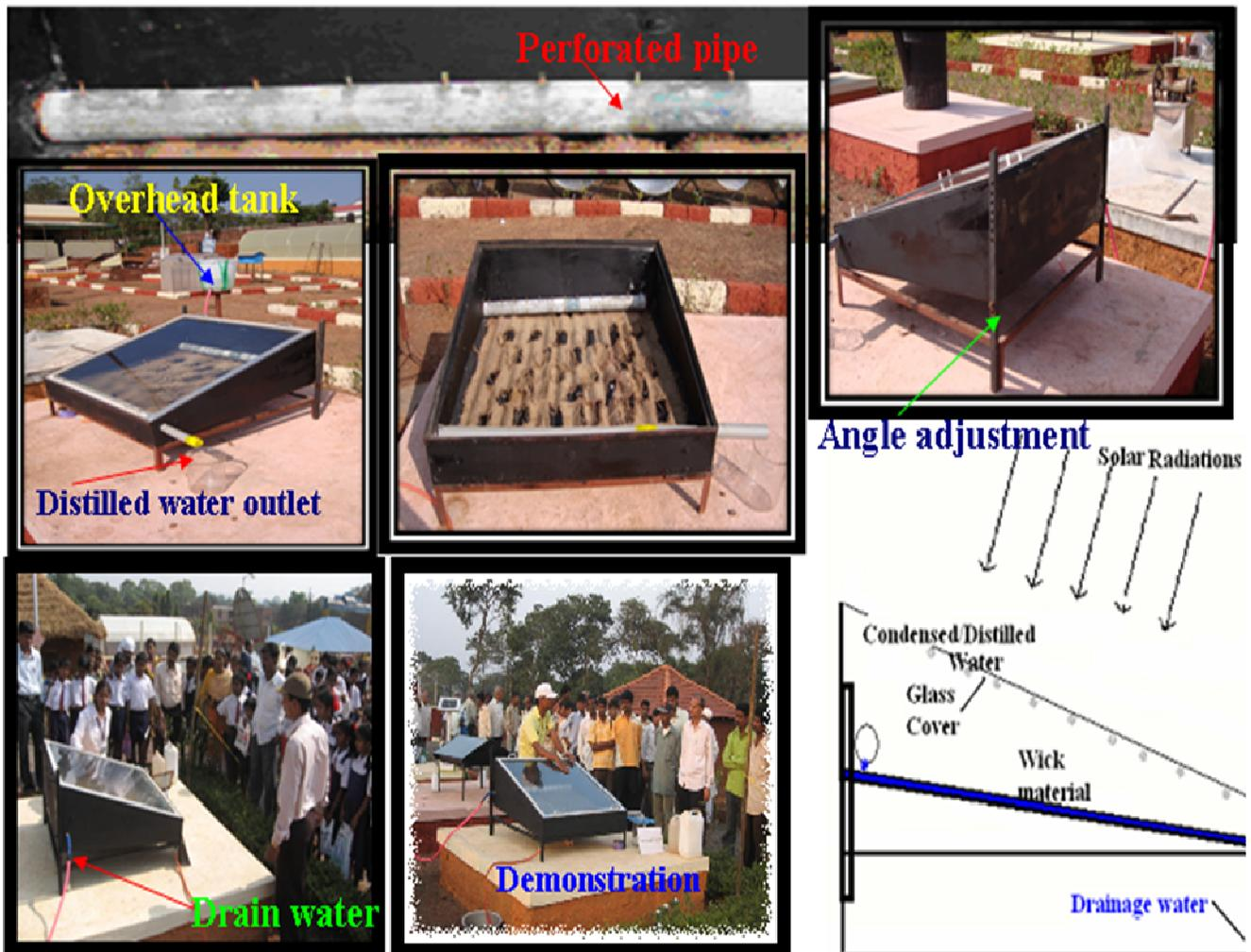
Figure 2. Single basin wick type solar distillation system.
