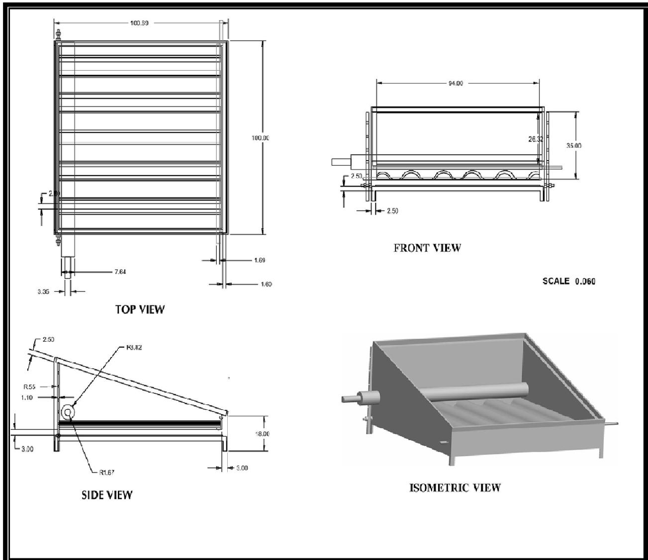
Figure 1. Constructional detail of SBWSD.
