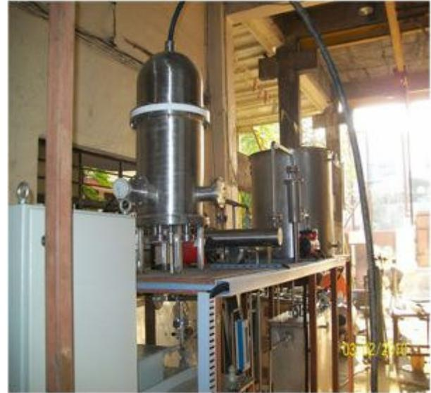
**Figure 9.** Photograph of the ozone generator cum processor.
