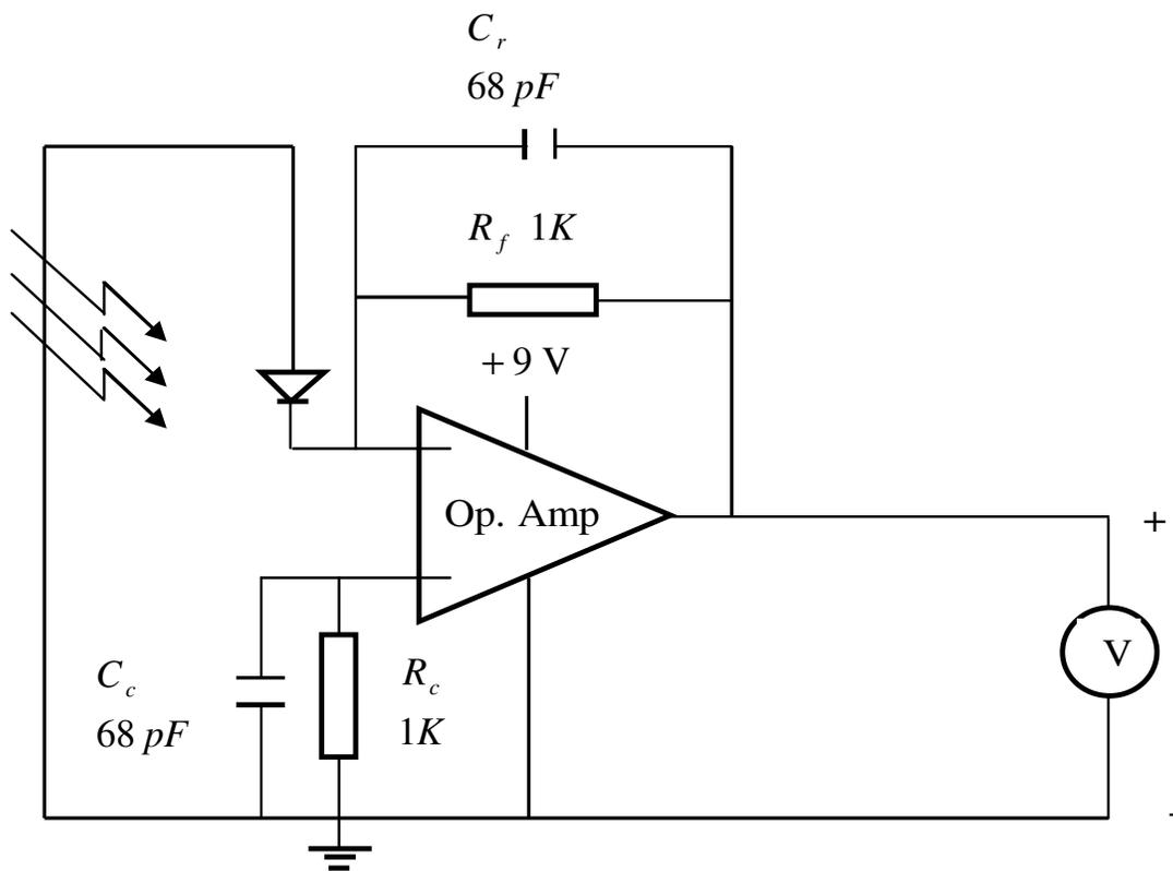
Figure 2. Pyranometer circuit diagram.
