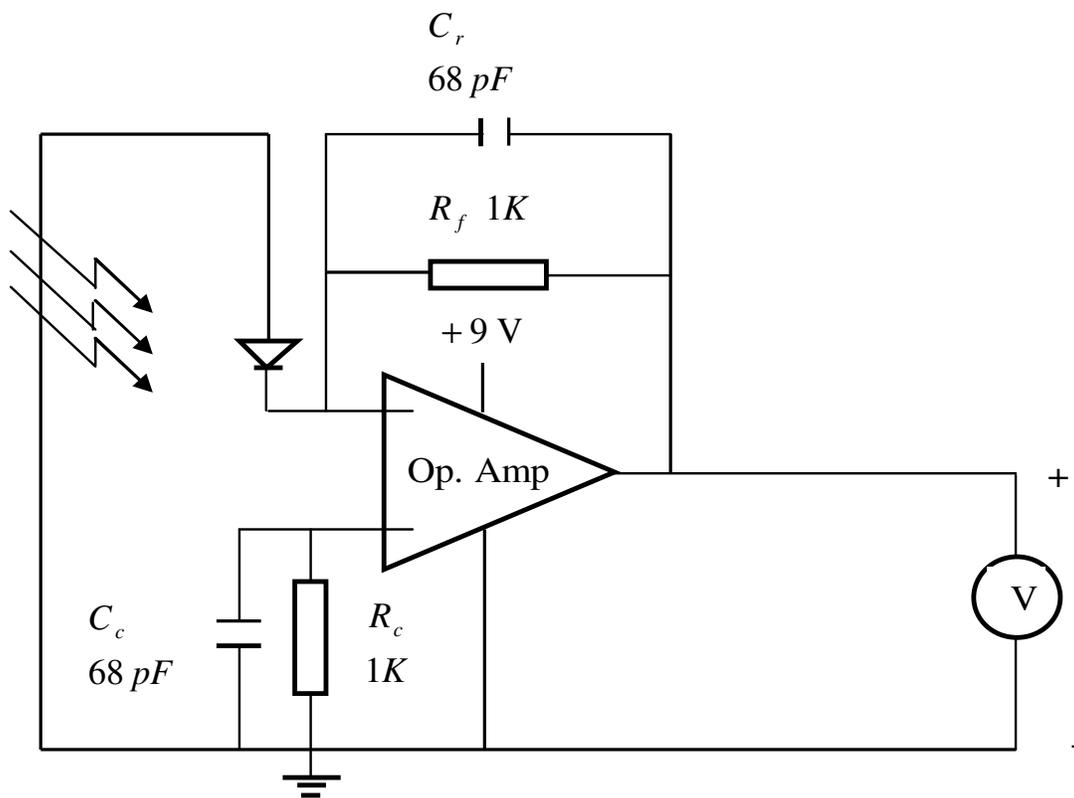
Figure 2. Pyranometer circuit diagram.
