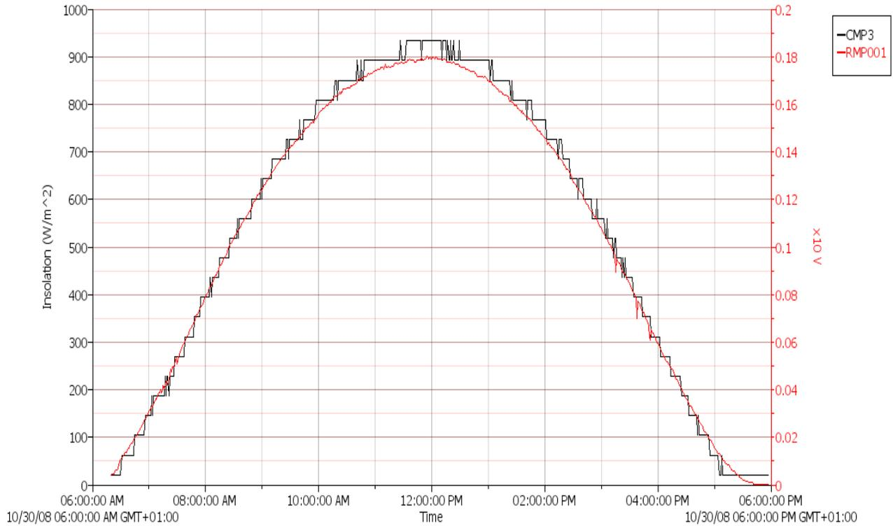
Figure 4. Graph of solar radiation measured with CMP3 and RMP001 versus time on 30<sup>th</sup> October, 2008.
