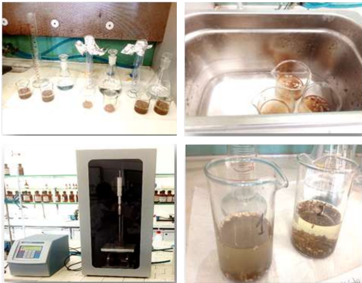
Figure 3. Ultrasound probe and bath extraction of Anacardic acids. Image obtained during extraction of the Anacardic acids in the laboratory. Source: Author
