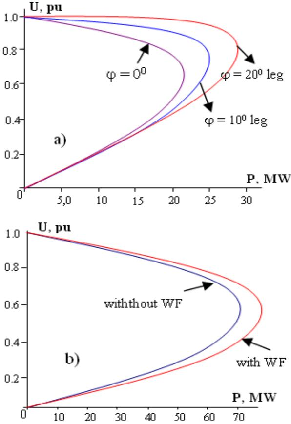
Figure 10. PV characteristics at PCC (a) and Phan Rý (b) under connected and unconnected WP condition.
