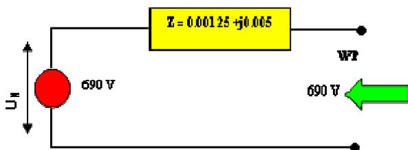
Figure 9. Equivalent grid and connection system impedance as seen from the low voltage (690 V).
