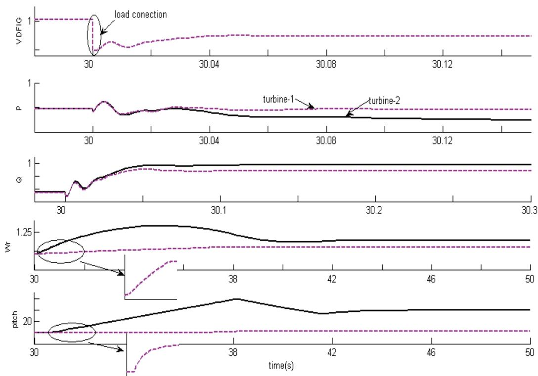
Figure 14. Turbine disconnection condition.
