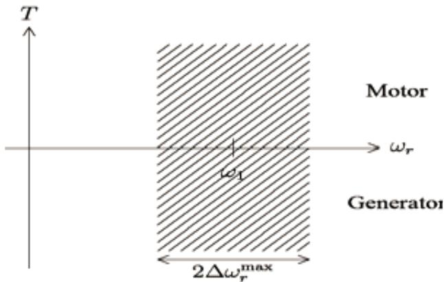
Figure 2. Speed torque characteristics of a DFIG.
