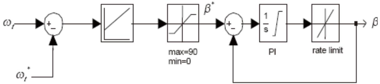
Figure 4. Pitch controller diagram.
