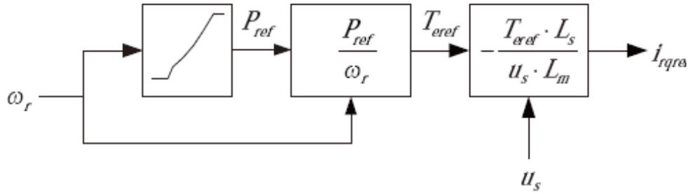
Figure 5. Active power control diagram.
