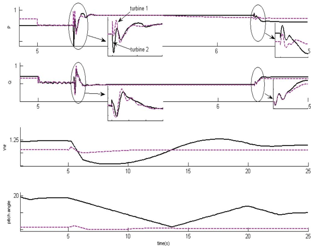
Figure 13. DFIG operation for three-phase fault condition.
