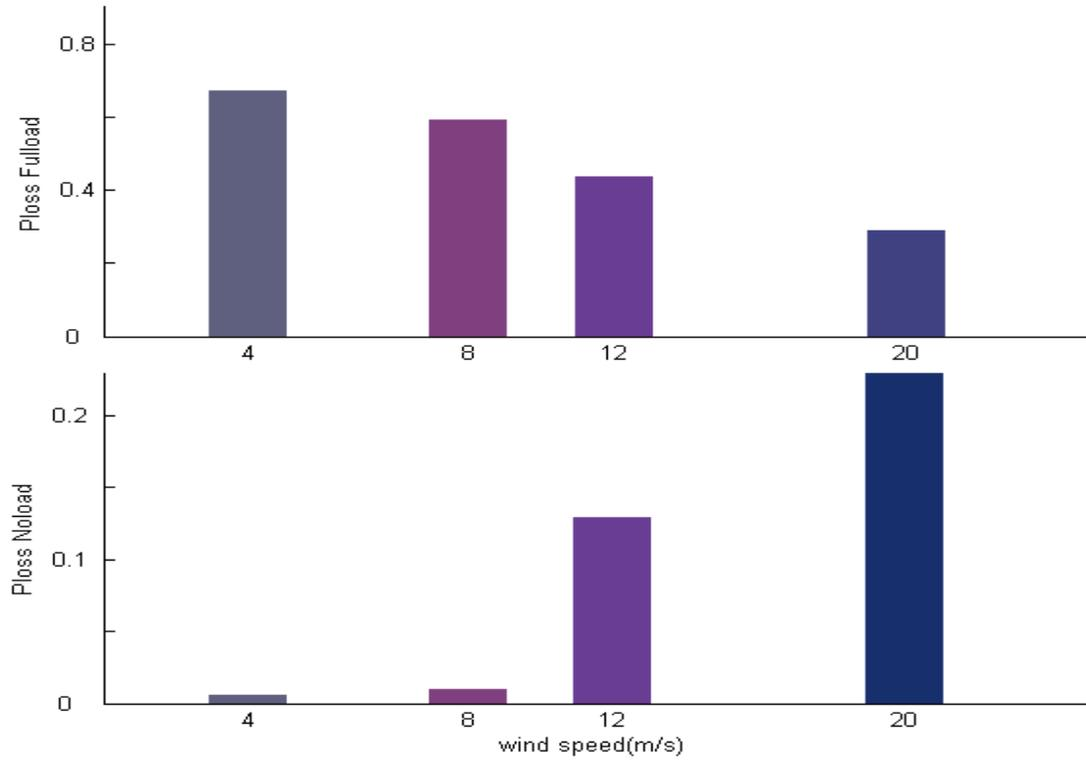
Figure 11. Active power losses at full load and no-load.
