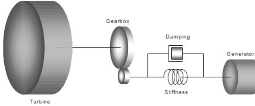
Figure 3. Drive- train system of WT-DFIG.
