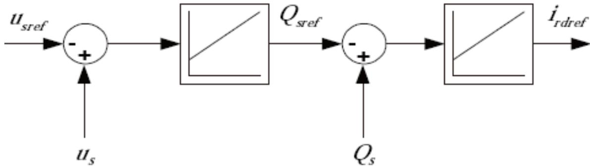
Figure 6. Reactive power and voltage control diagram.
