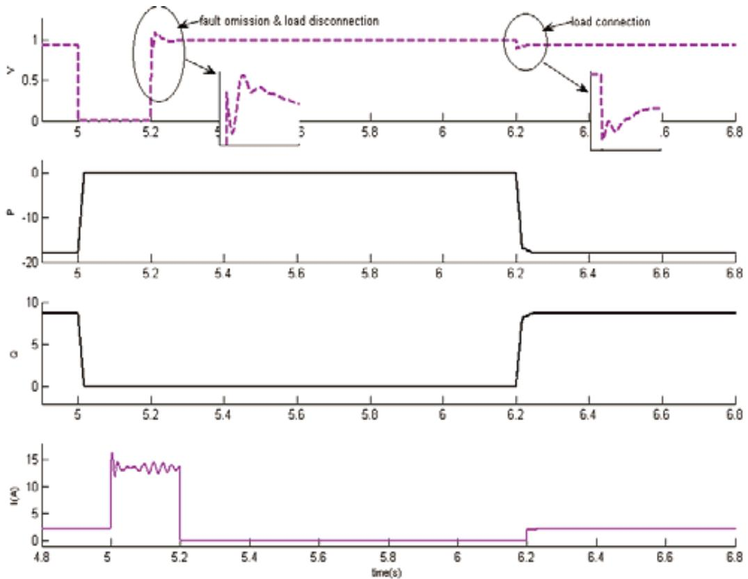
Figure 12. Three-phase fault on the load bus.
