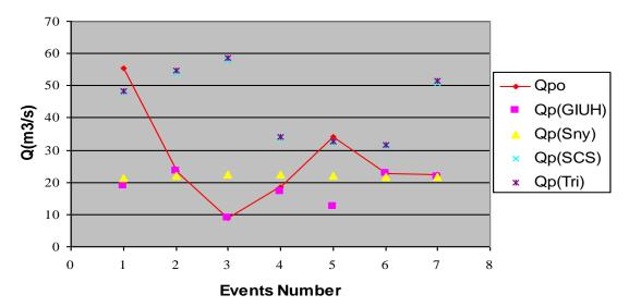
Figure 6. Observed discharge and peak discharge estimation from using models.
