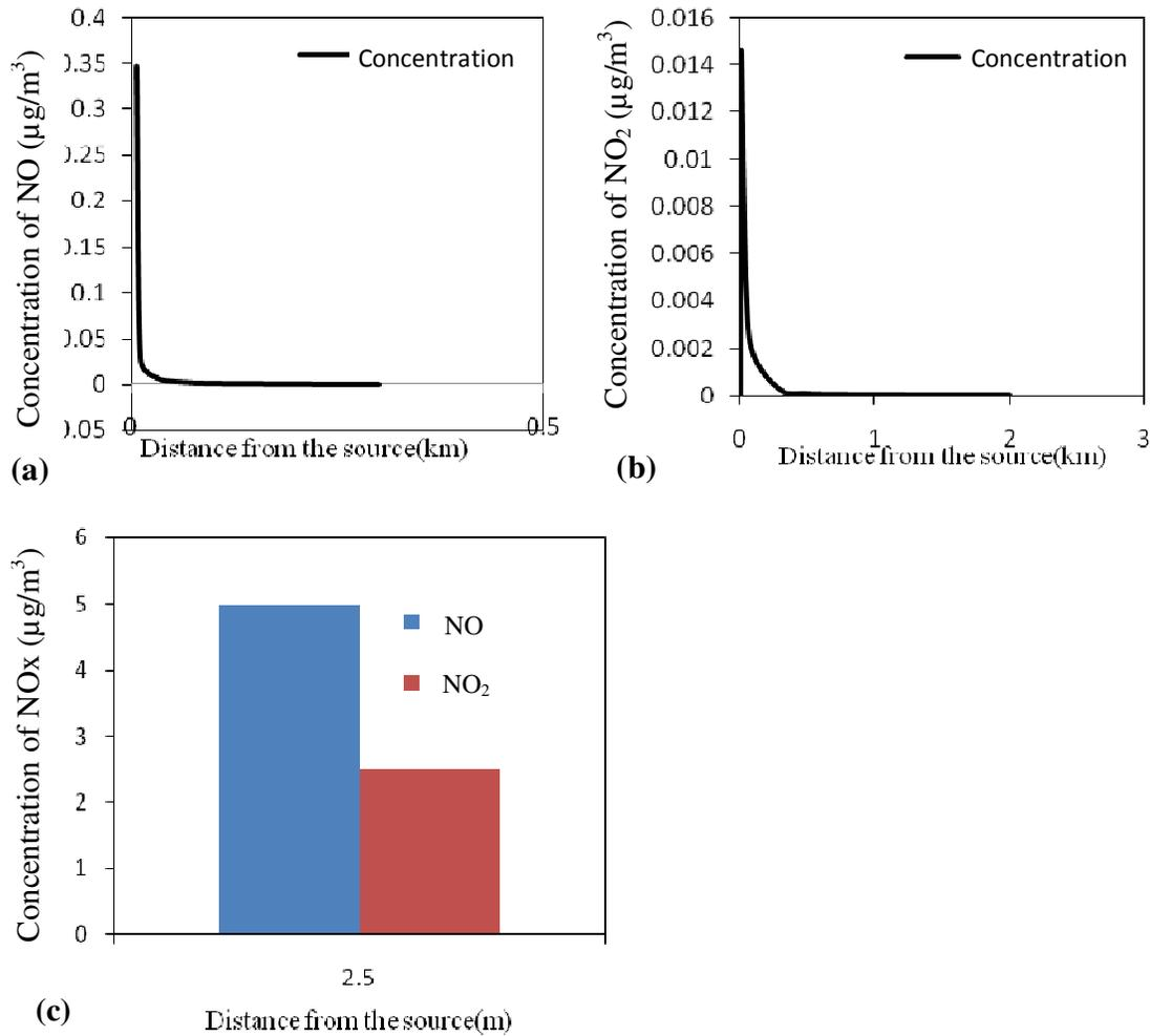
**Figure 11.** (a) The modeled NO conc. with distance (b) the modeled NO<sub>2</sub> conc. with distance (c) the measured NOx concentration with distance.
