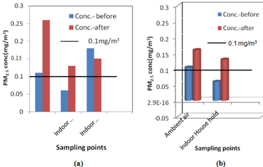
**Figure 22.** A comparison of the ambient PM<sub>2.5</sub> from the horizontal (a) and vertical (b) stacks.
