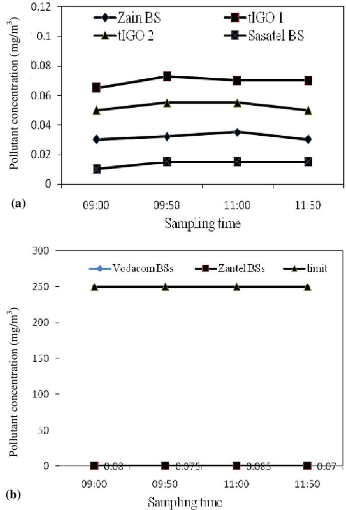
**Figure 10.** (a) Stack NO<sub>2</sub> emissions for different generator (b) NO<sub>2</sub> concentration against the stack emission standard 250 mg/m<sup>3</sup>.
