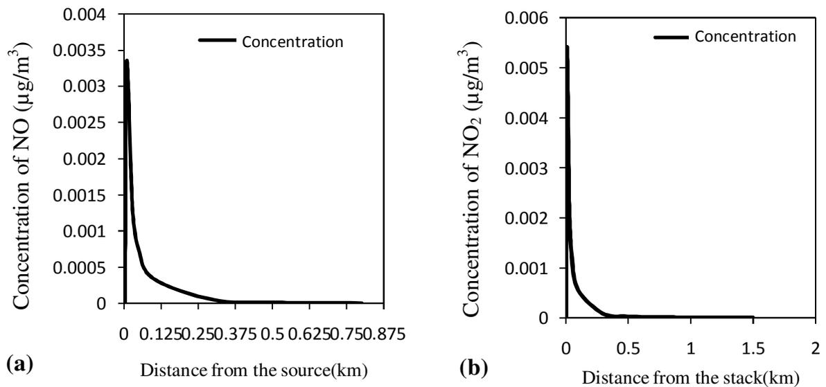
**Figure 12.** (a) Modeled NO concentration for Sasatel tower (b) Modeled NO<sub>2</sub> conc. for Sasatel tower.
