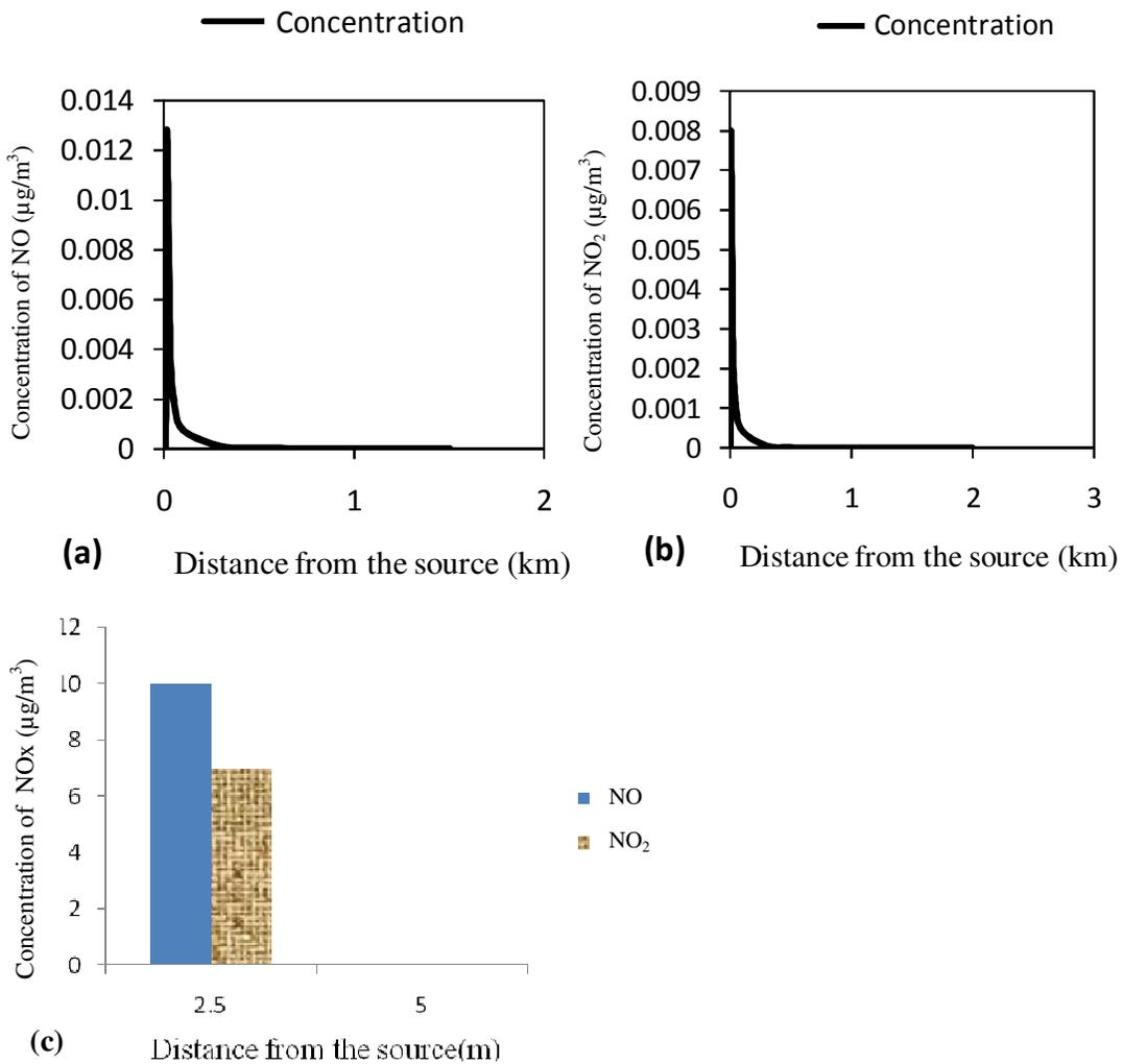
Figure 15. (a) Modeled concentration of NO for Zain tower (b) Modeled concentration of NO<sub>2</sub> for Zain BS (c) The measured NOx concentration with distance.
