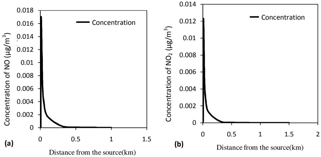
Figure 14. (a) Modeled conc. of NO for Zantel (b) Modeled conc. of NO<sub>2</sub> for Zantel.
