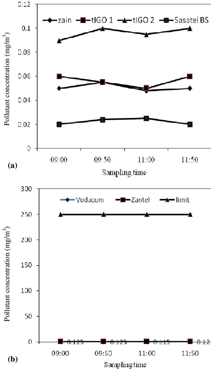
**Figure 9.** (a) Stack NO emissions for different generator stacks (b) NO concentration against the stack emission standard of 250 mg/m<sup>3</sup>.
