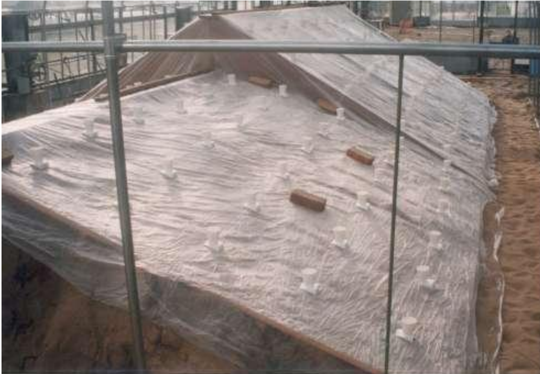
Figure 3. Setup for measuring uniformity and spray characteristics of overhead rainfall system (cups collect rain water).
