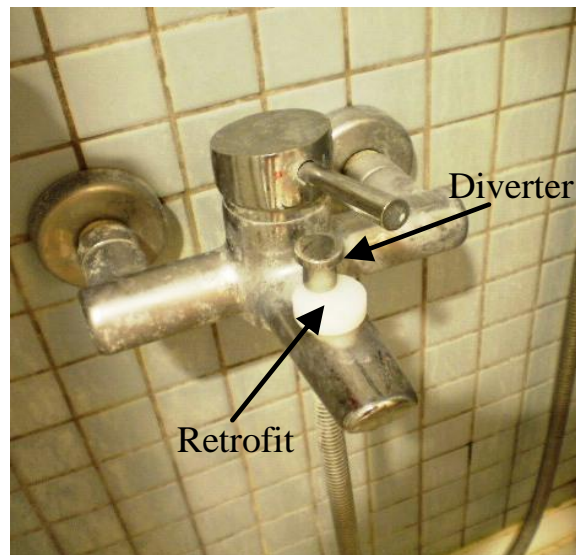
Figure 3. A photograph from the test of the retrofit, retrofit keeps the diverter at its up-position.
