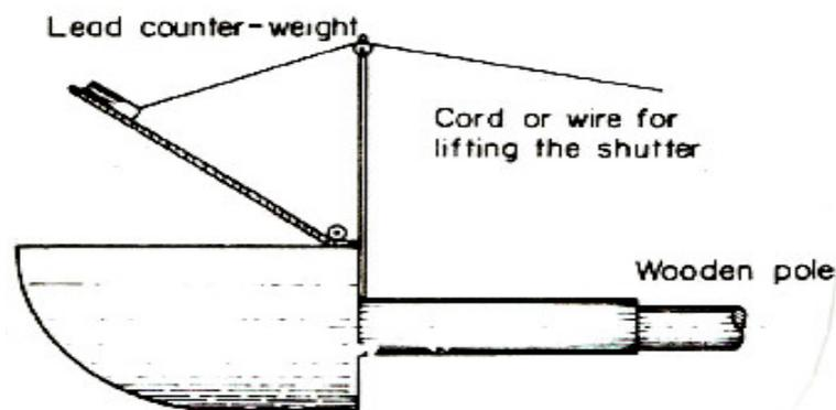
**Figure 2.** Scoop sampler with shutter.
