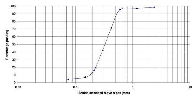
Figure 4. Particle size curve for Goruba River bed material.
