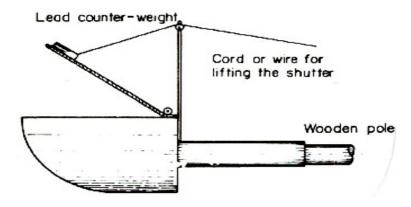
Figure 2. Scoop sampler with shutter.
