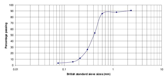
Figure 3. Particle size curve for Samaru River bed material.
