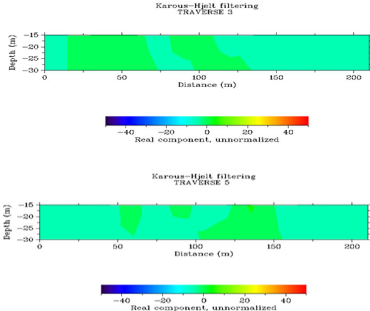
**Figure 2b.** Sample Karous-Hjelt filter 2-D inversion current density sections (Traverses 1, 3 and 5).
