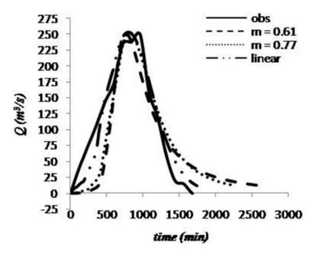
**Figure 6.** The estimated and observed hydrographs for the storm which occurred on 7th January, 2002 in the Rood Zard catchment.
