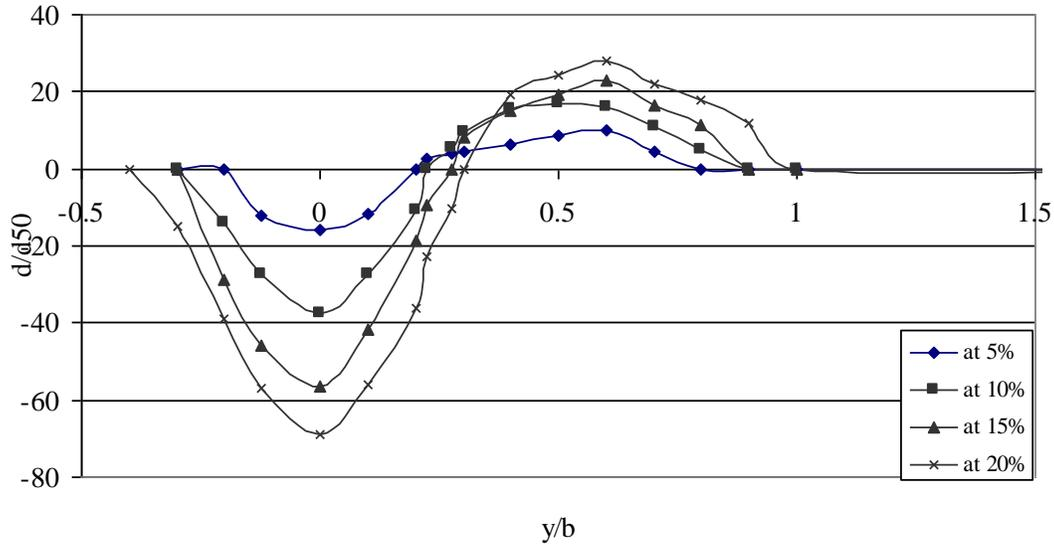
Figure 6. Longitudinal profiles of the scouring depth  $d$ , for different grain lengths ( $\alpha = 90^\circ$ ).
