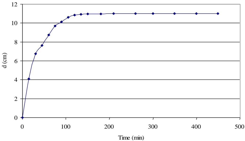
Figure 2. Curve for balance time (groin 8 cm and 90° groin inclination angle).
