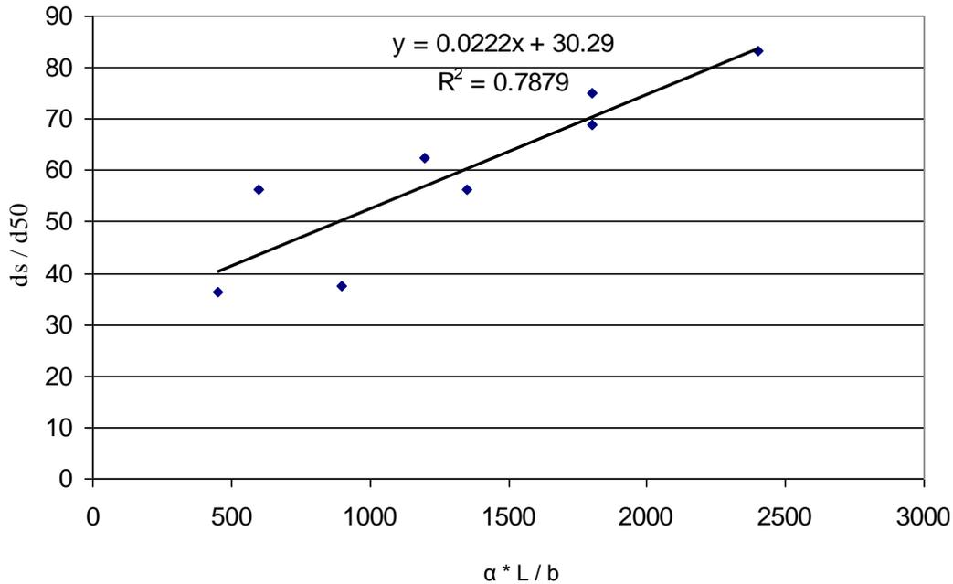
**Figure 10.** Effect of the 8 cm- groin angle of inclination on the maximum scouring depth.
