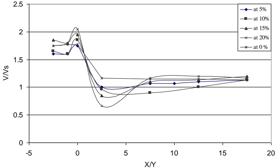
Figure 3. Longitudinal velocity distributions for different groin lengths ( $\alpha = 90^\circ$ ).
