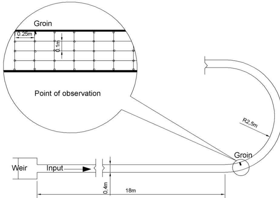
Figure 1. The laboratory layout of the experimental flume.
