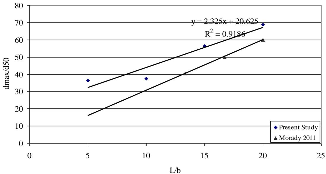
Figure 7. Comparison of present study and Moradi results for effect of grain length on the maximum scouring depth ( $\alpha = 90^\circ$ ).
