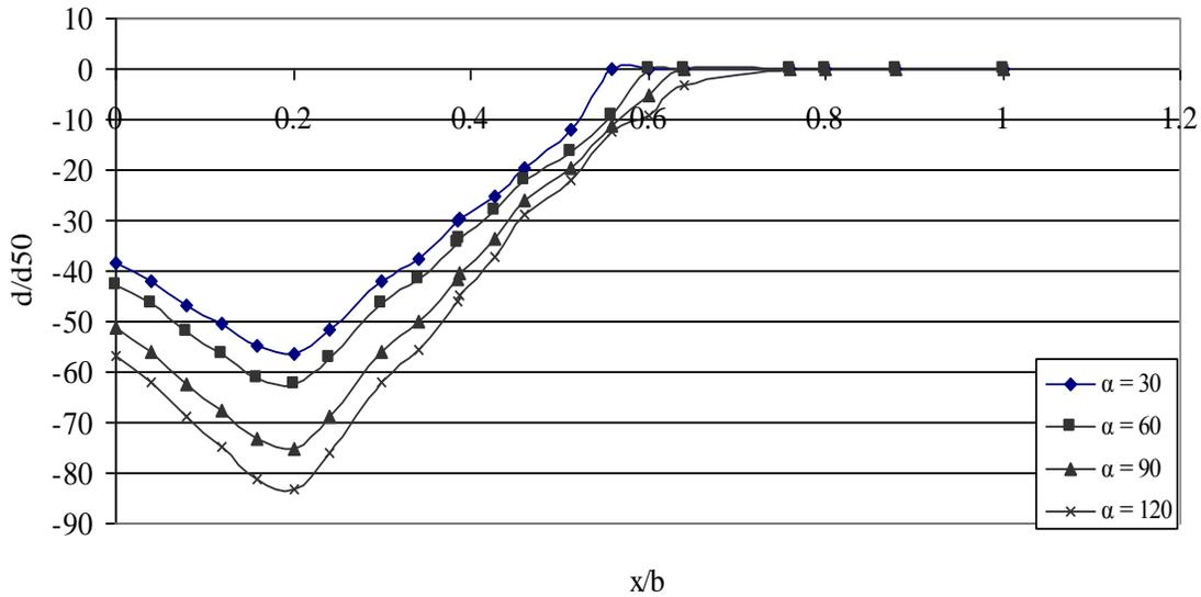
**Figure 8.** Transverse profiles of 8 cm - groin for different inclination angle.
