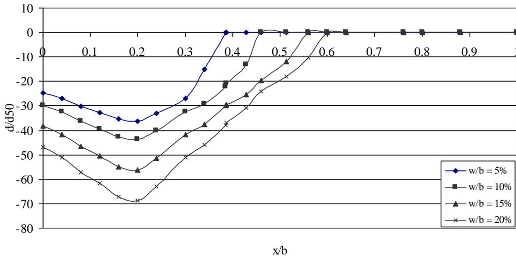
Figure 5. Latitudinal profiles of the scouring depth d, for different groin lengths ( $\alpha = 90^\circ$ ).
