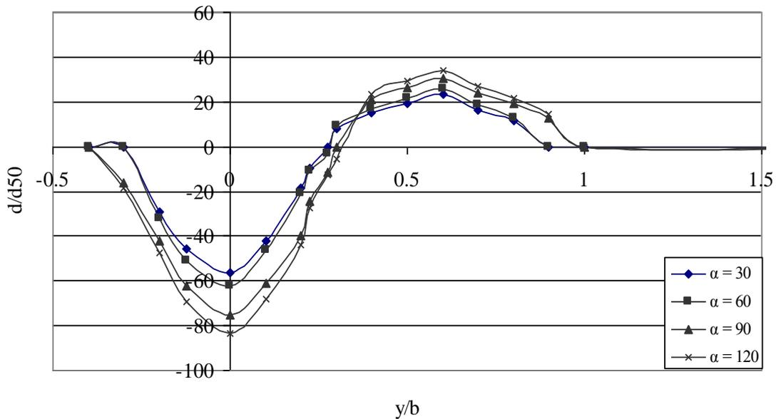
**Figure 9.** Longitudinal profiles for different the 8 cm groin inclination angle.
