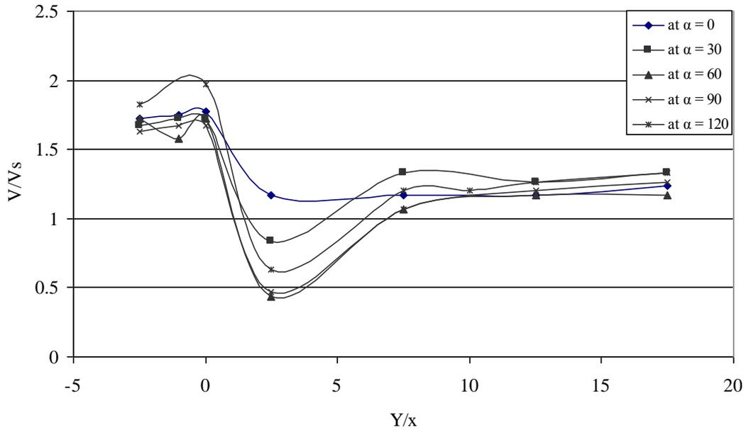
Figure 4. Variations of velocity distributions due to the 8 cm groin angle of inclination.
