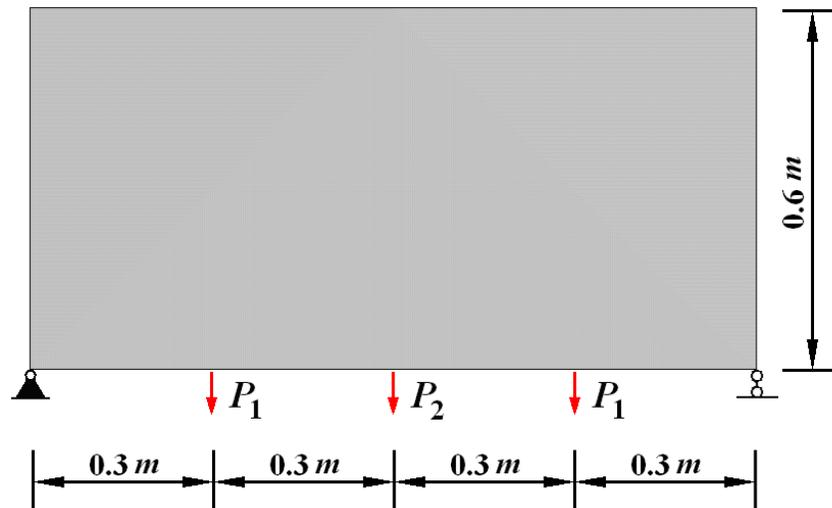
Figure 4. Initial design domain of structure.
