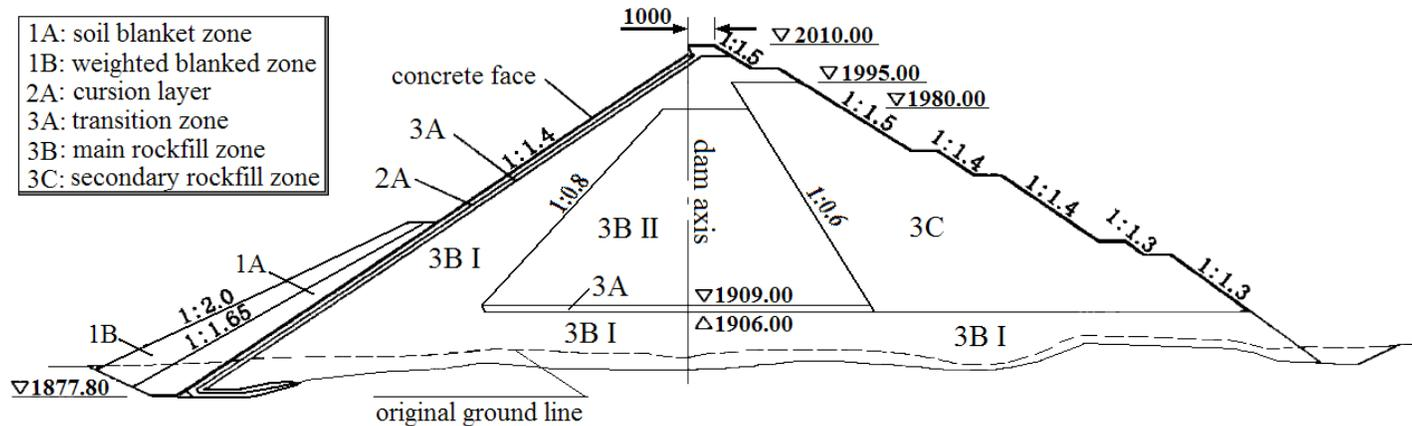
Figure 1. Section of Gongboxia dam (CFRD in Qinghai, China).
