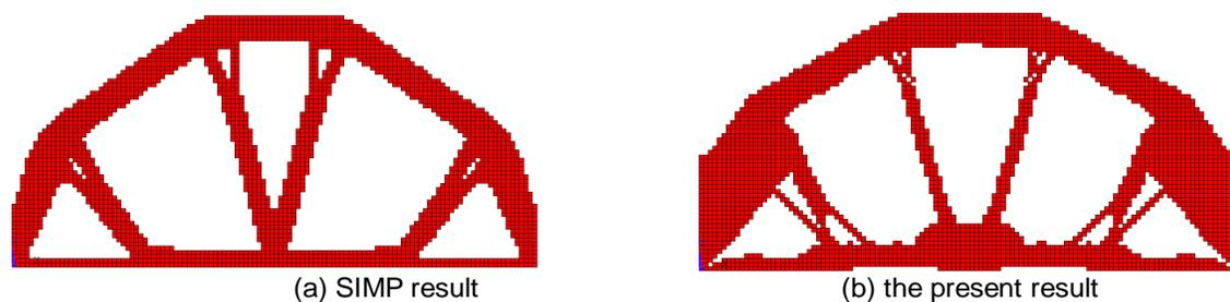
**Figure 5.** Biphase layout optimization results by different methods (the red represents stiffer material and the rest is softer material).
