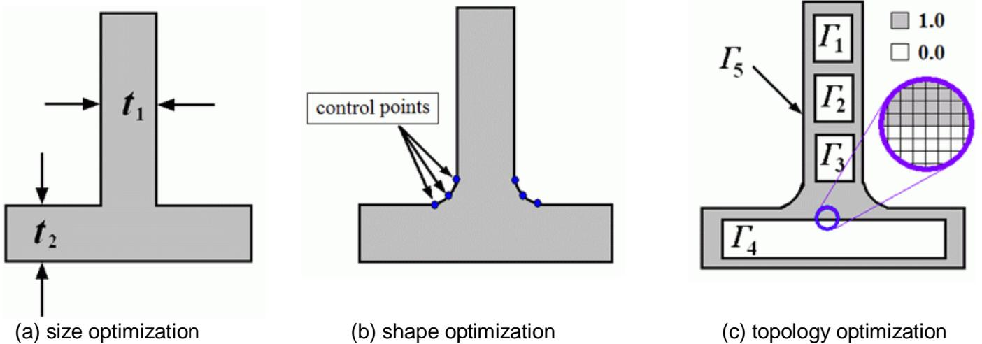
**Figure 2.** Differences between size optimization, shape optimization and topology optimization, (a) size optimization with design variables (DVs) of  $t_1$  and  $t_2$ , (b) shape optimization with DVs of positions of control points on boundary, (c) topology optimization is to find the boundaries of structure.
