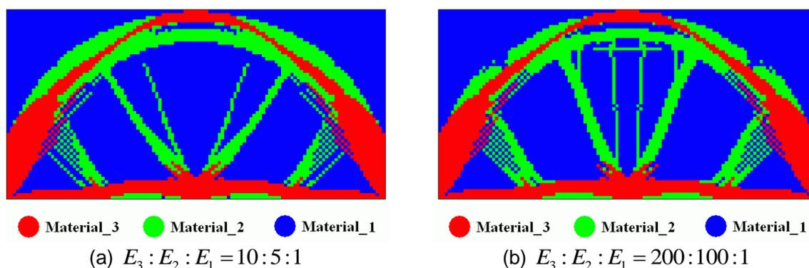
**Figure 6.** Optimized material distributions for the two cases. (Material 3 with  $E_3$ , Material 2 with  $E_2$  and Material 1 with  $E_1$ ).
