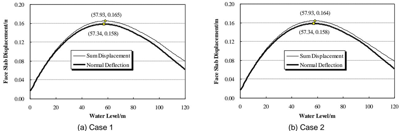
Figure 10. Deflections of face slab for two cases.
