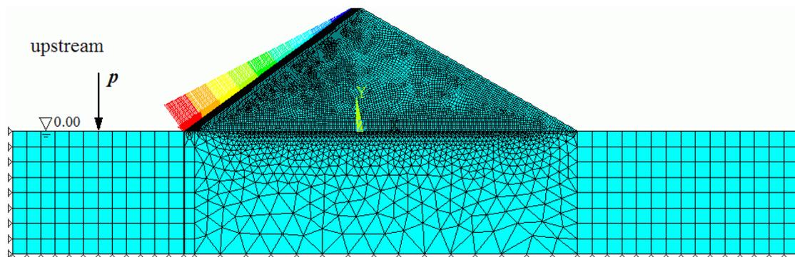
Figure 7. Finite element model of dam and foundation.
