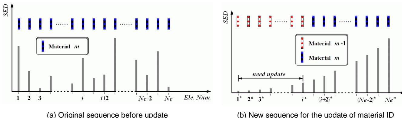
**Figure 3.** Sorting of the SEDs of elements with Material  $m$  in design domain: (a) initial number sequence of elements with material  $m$  only and (b) ascending order of the values of SEDs of elements with either material  $m$  or  $m-1$ .
