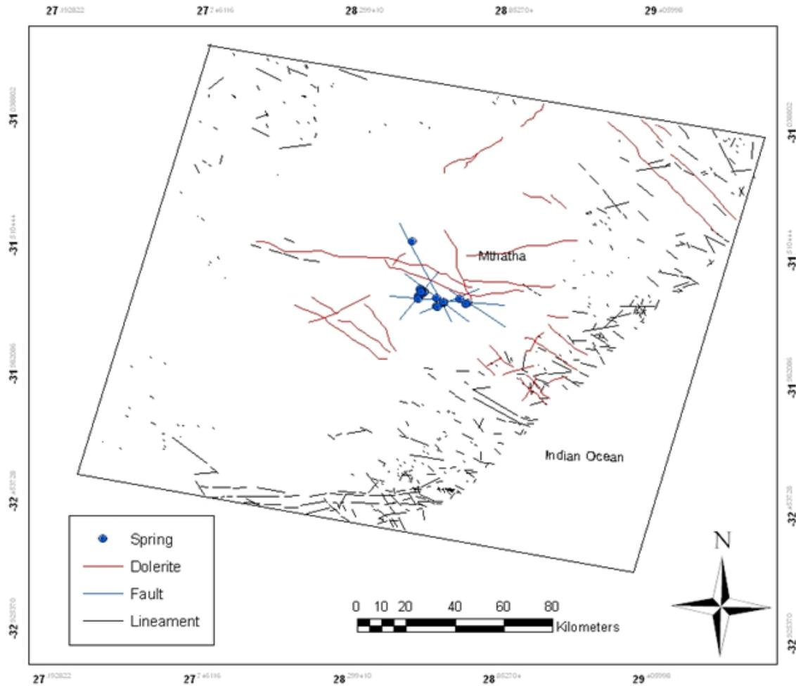
**Figure 8.** Lineaments extracted from satellite image 169/082.
