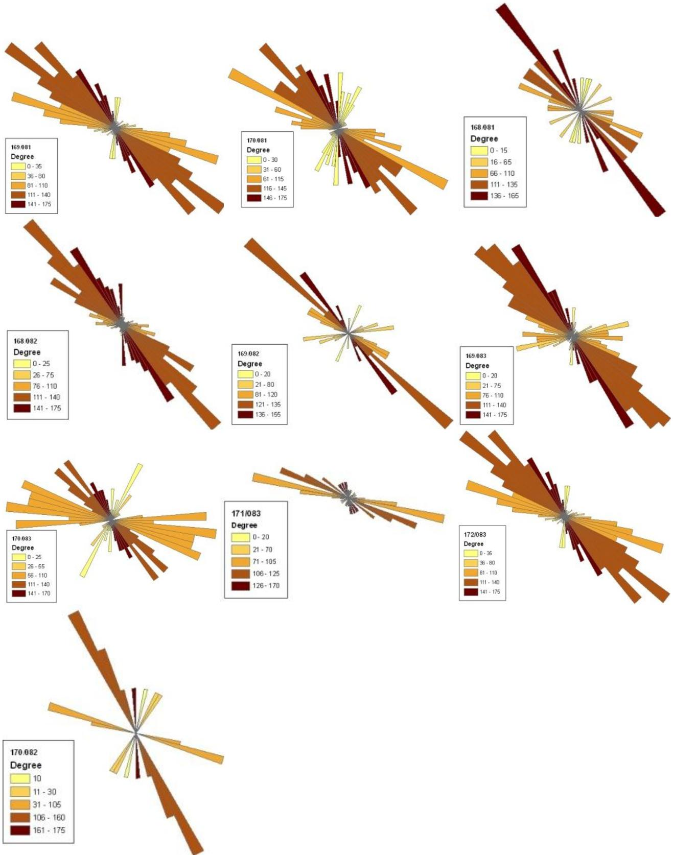
Figure 16. Rose plots derived from the lineament maps in the neotectonic belts.
