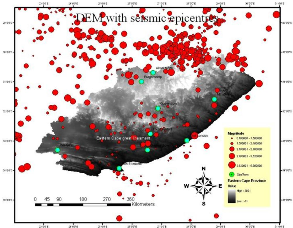
**Figure 11.** Digital elevation model of the Eastern Cape Province, the great lineament has seismic epicenters within it.
