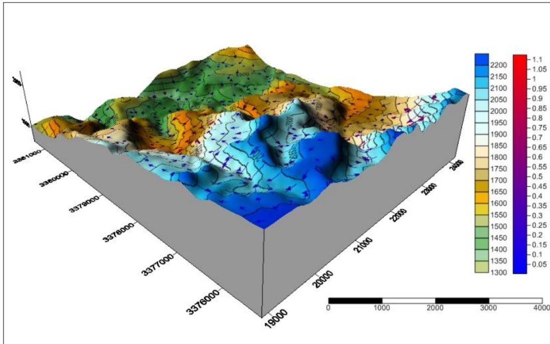
**Figure 20.** Digital elevation model sample and vector gradients of Grid 3028DB.
