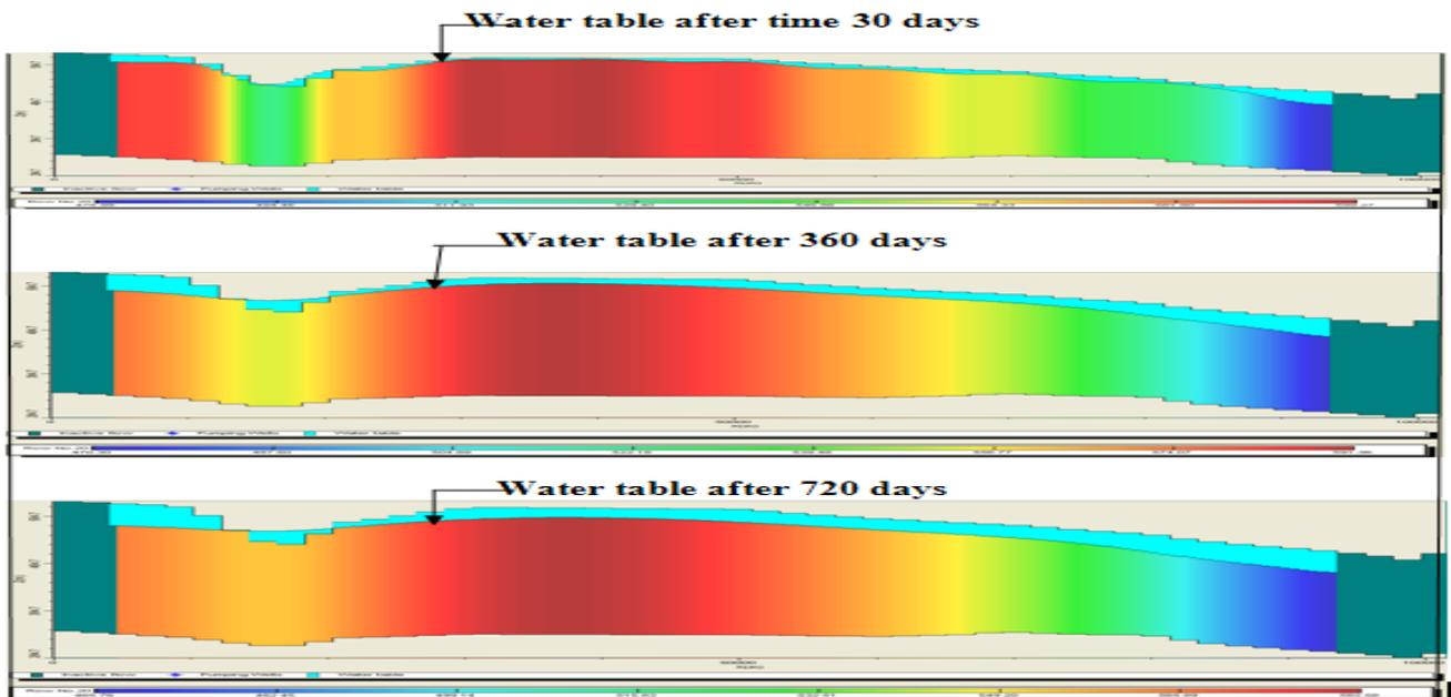
Figure 6. Cross-sections present the falling in water table during the calibration period (2008-2009).
