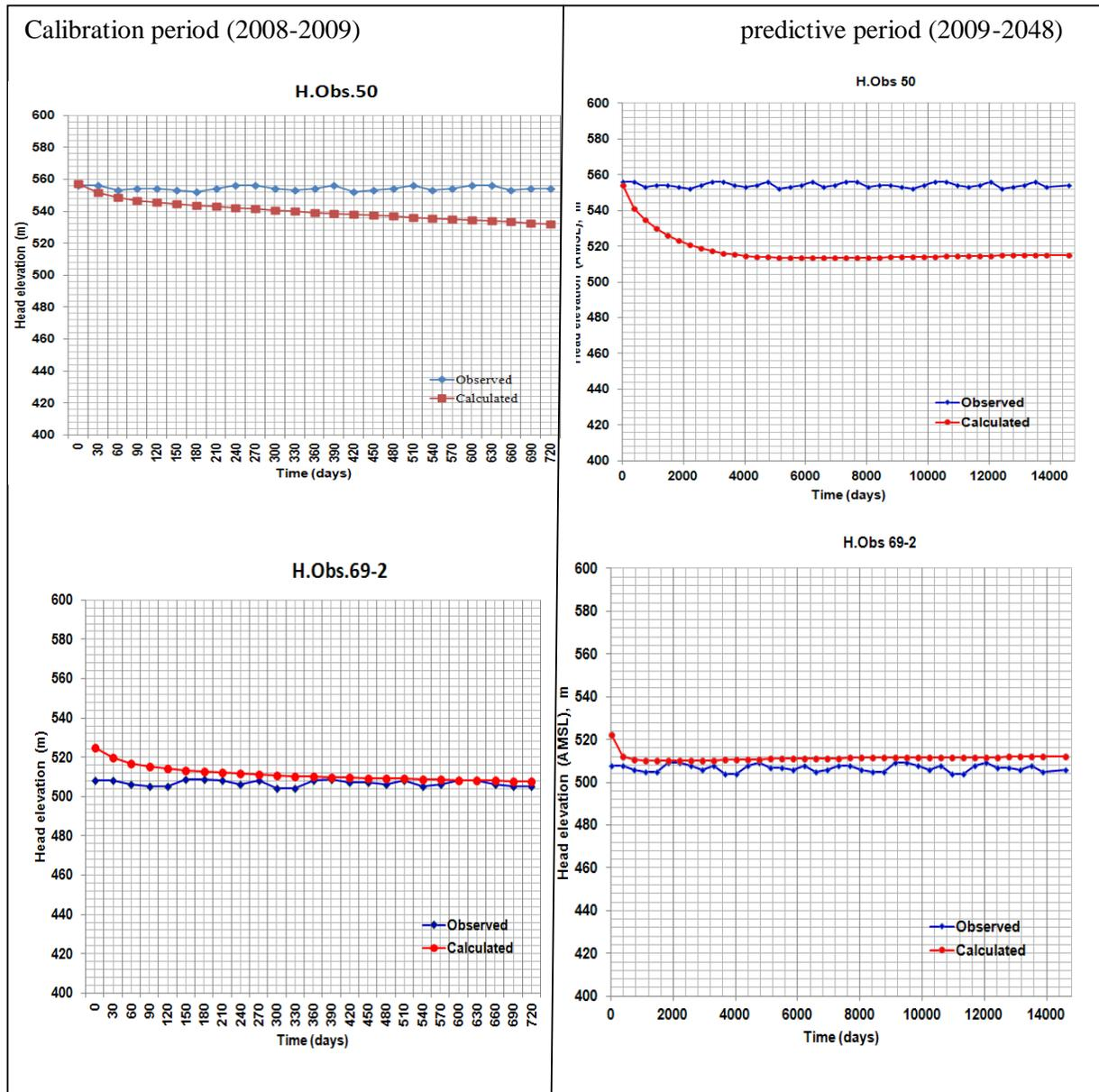
**Figure 8a.** Illustrated the head elevation during the calibration and predictive period for head observations .H.obs.50 and H.Obs.69-2
