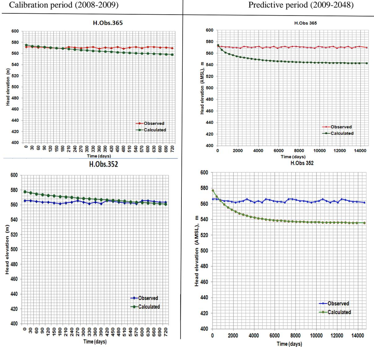
**Figure 8b.** Fit the head elevation during the calibration and predictive period for head observations .H.obs.365 and H.Obs.352.
