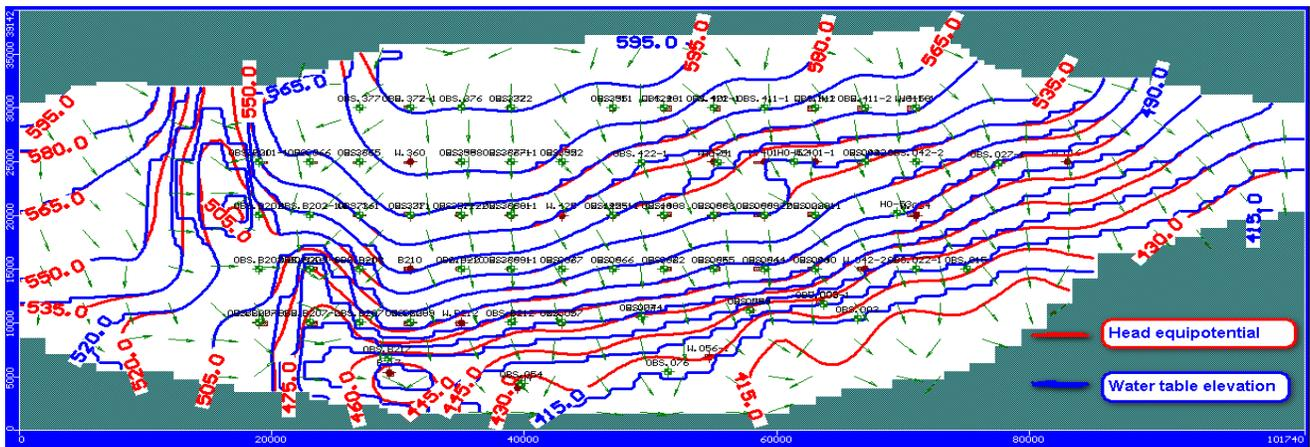
Figure 7. Map showing the velocity direction of groundwater in the domain and comparison between the simulated and the observed head, the observed is appear as red ,while the blue is the calculated.
