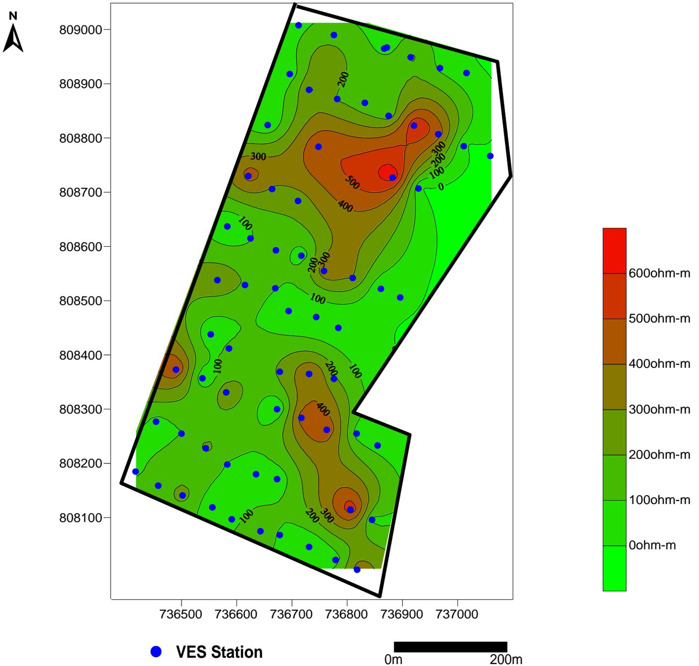
Figure 9. Isoresistivity of the weathered layer.
