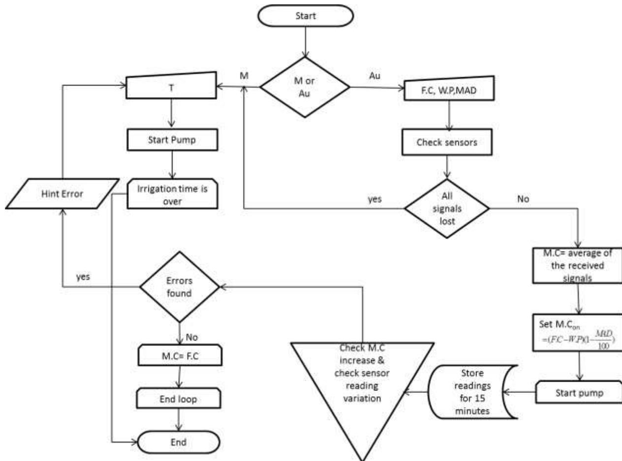
Figure 3. Flow chart of the control system's software.
