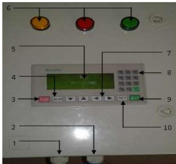
**Figure 1.** Control system containing box and interface components. 1- Control unit power input cable path, 2- Sensors signal and pump power cables path, 3- Escape button to get out of a menu, 4- Check errors button (ALM), 5- Digital screen, 6- Sensors' signals indicator, 7- Transfer buttons, 8- Numeric input buttons, 9- Data Entry confirmation button, 10- Input and system settings menu button.
