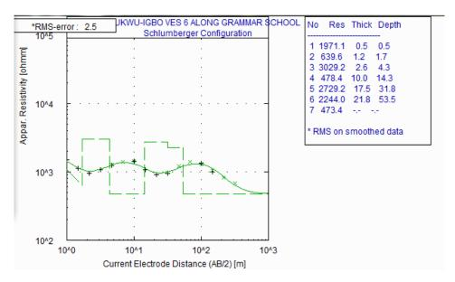
Figure 6. Typical Sounding Curve for Akwukwu-Igbo (VES 6) HKHKQ - curve type.
