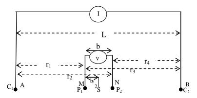
**Figure 2.** Schlumberger field electrodes configuration. Where "L" is the distance between the current electrodes and "b" is the distance between potential electrodes in station S.
