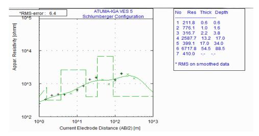
Figure 5. Typical Sounding Curve for Atuma Iga (VES 5) QKHK - curve type.
