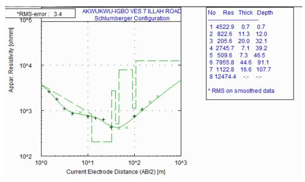
Figure 7. Typical Sounding Curve for Akwukwu-Igbo (VES 7) QHKHA - curve type.
