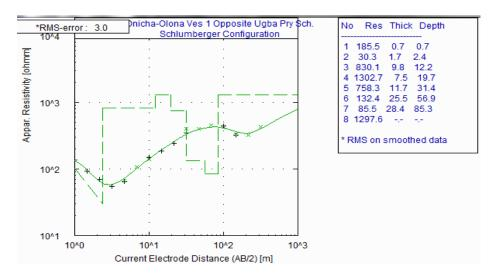
Figure 3. Typical Sounding Curve for Onicha Olona (VES 1) HAK - curve type.
