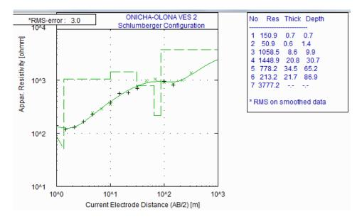
Figure 4. Typical Sounding Curve for Onicha Olona (VES 2) HAH - curve type.
