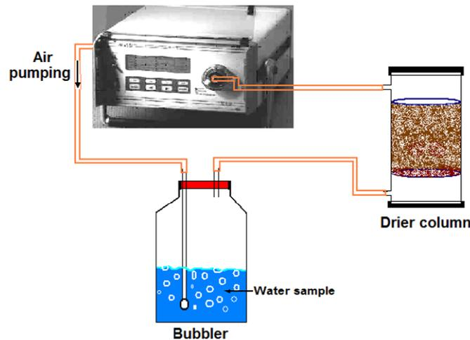
**Figure 2.** The PRASSI system set up for radon measuring in the water sample.
