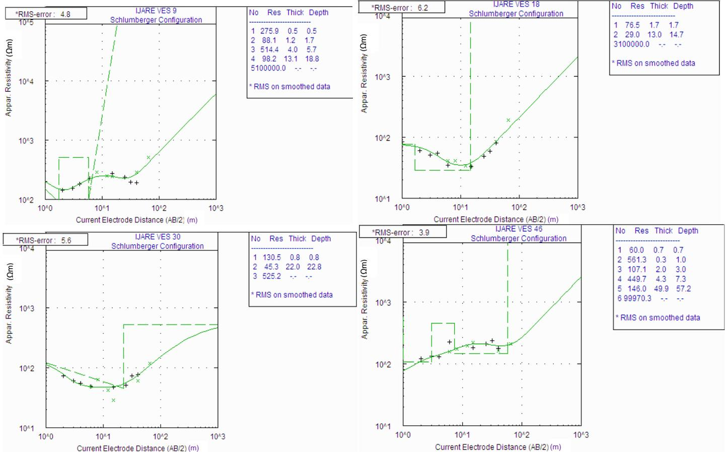
Figure 4. Typical geo-electric sounding curves obtained from Ijare town.
