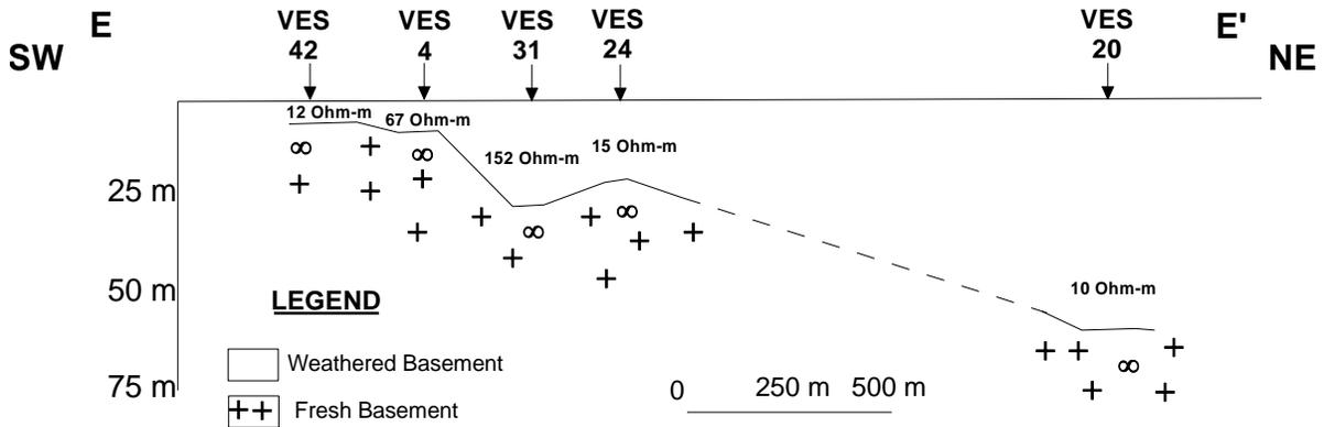
Figure 9. Geoelectric section along profile E-E'.
