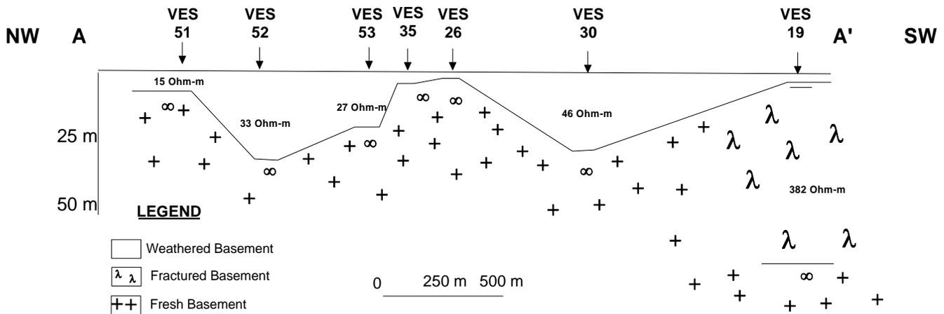
Figure 5. Geoelectric section along profile A-A'.
