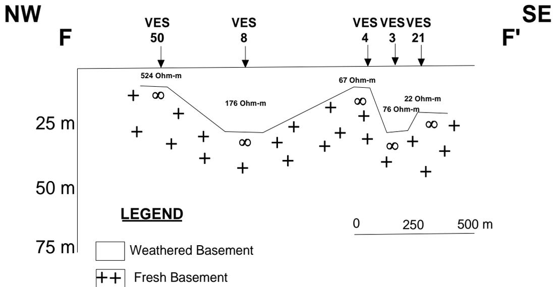
Figure 10. Geoelectric section along profile F-F'.
