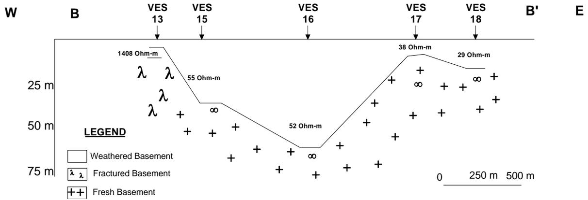
Figure 6. Geoelectric section along profile B-B'.
