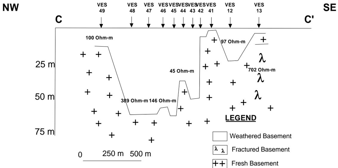
Figure 7. Geoelectric section along profile C-C'.
