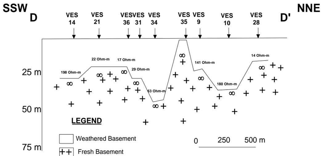
Figure 8. Geoelectric section along profile D-D'.
