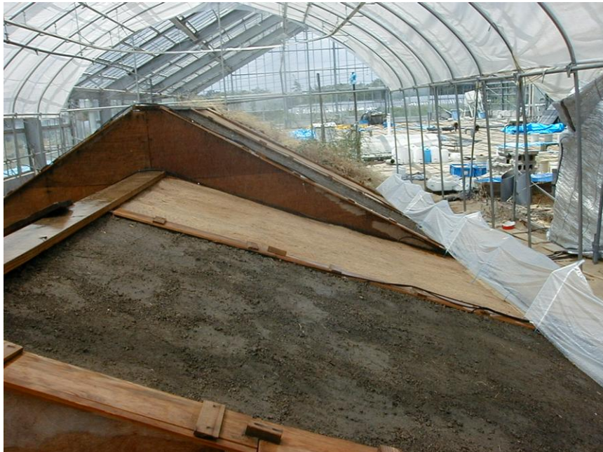
Figure 5. Rainfall-runoff experimental layout showing slopes with different top layer soil treatments.
