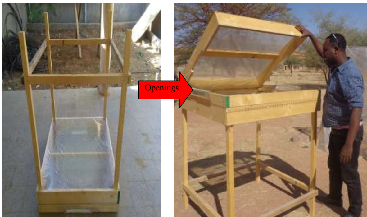
Figure 2. Raised rack tent dryer.
