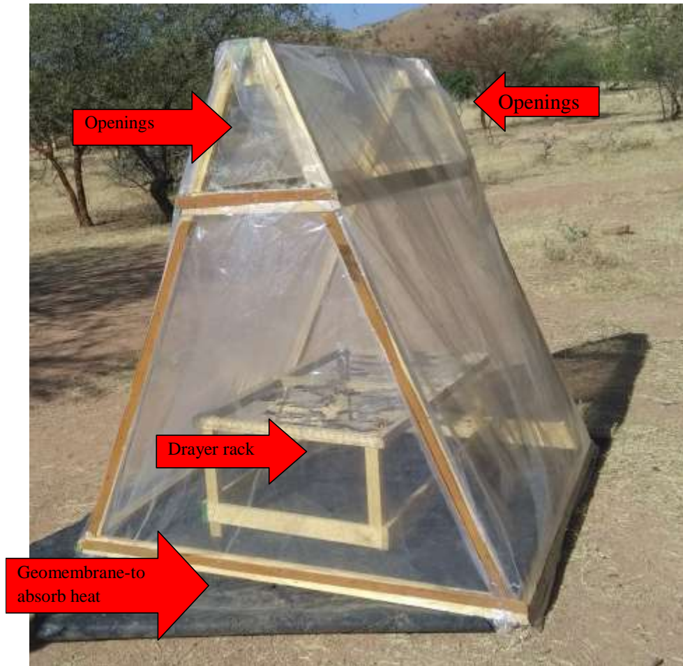
Figure 1. Solar tent dryer.
