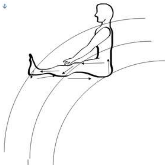
Figure 19. Sitting on one's buttocks is not risk free. There are dips underneath the knees. Current paths are shown by arrows.
