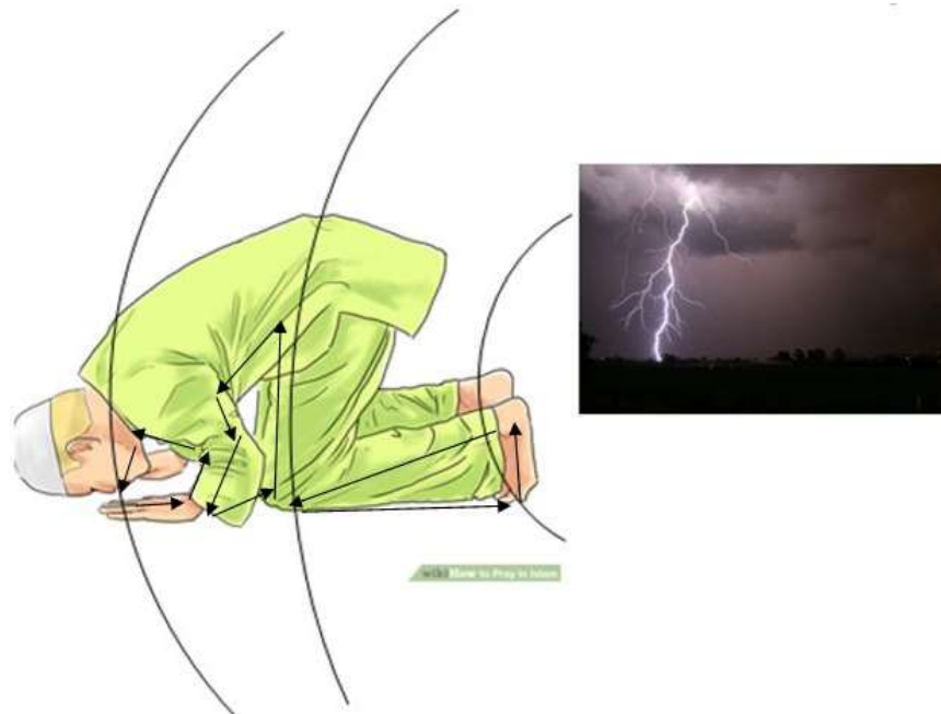
Figure 21. Muslim prayer position shortens the inter-limb distances and reduces the height offering the best protection from lightning. (Prostration picture taken from http://www.wikihow.com/Pray-in-Islam ).
