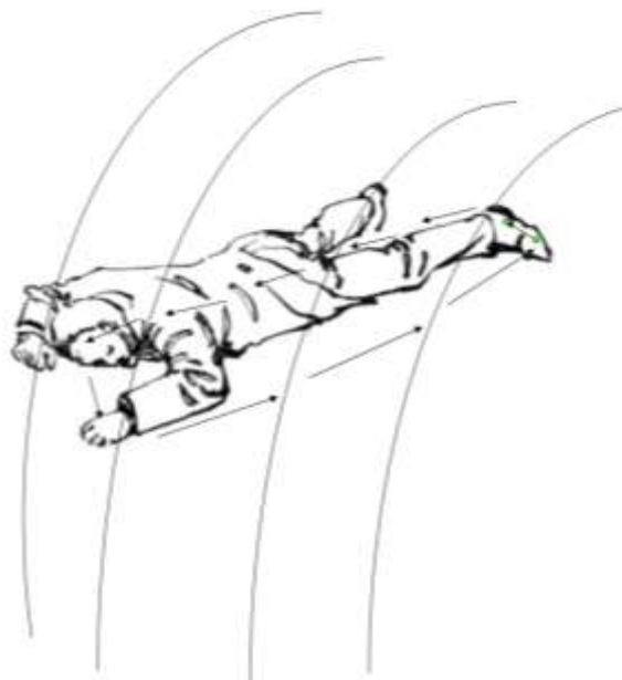
Figure 20. Lying down on the chest is dangerous. Ground could be uneven and there is a big dip below the abdomen. Lying down on the back is risky, too, because of the unevenness around the waist.
