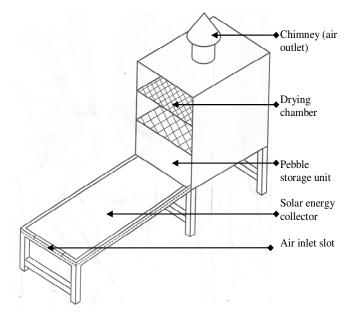
Figure 1. Laboratory-scale passive solar grain dryer.
