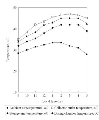
Figure 2. Typical plot of daily dryer system temperatures during the drying period.
