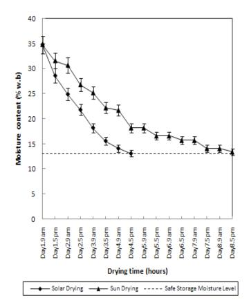
Figure 3. Variation of mean moisture content with drying time.
