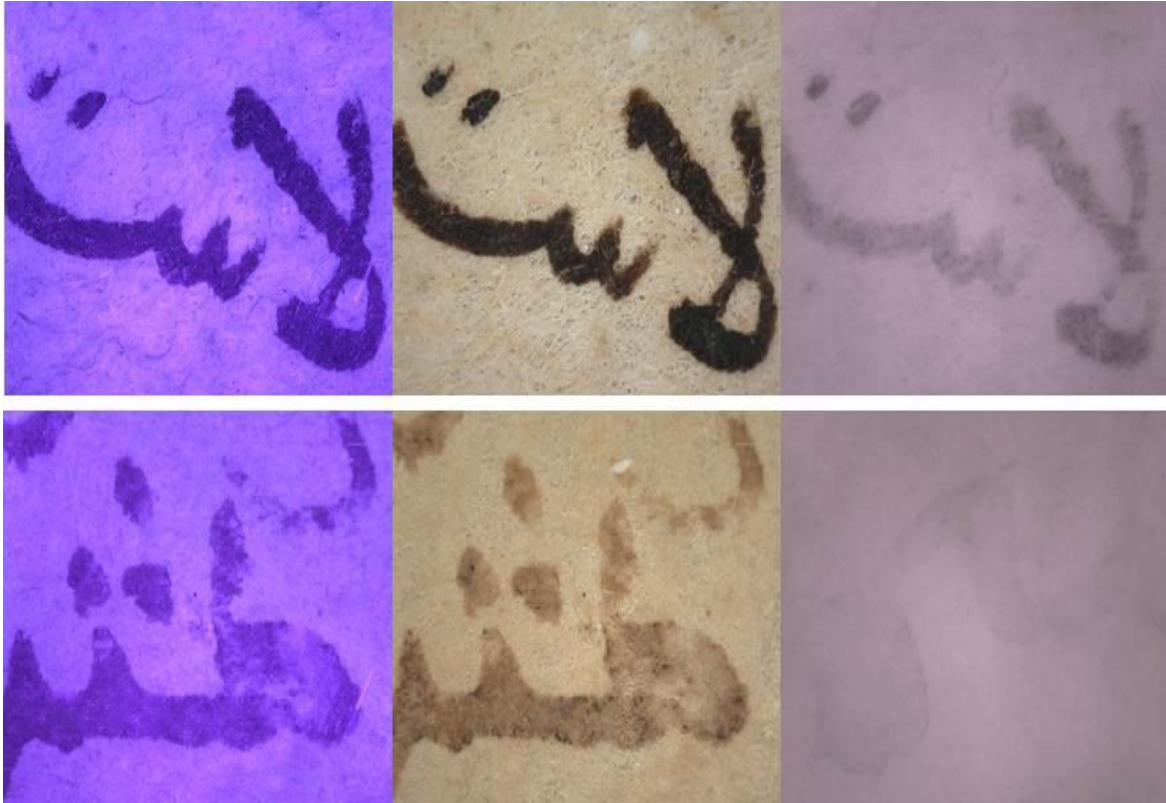
Figure 13b. Iron-gall ink of the comment (top row), iron-gall ink of the title (bottom row). The columns correspond to UV, VIS, and NIR illuminations, respectively.
