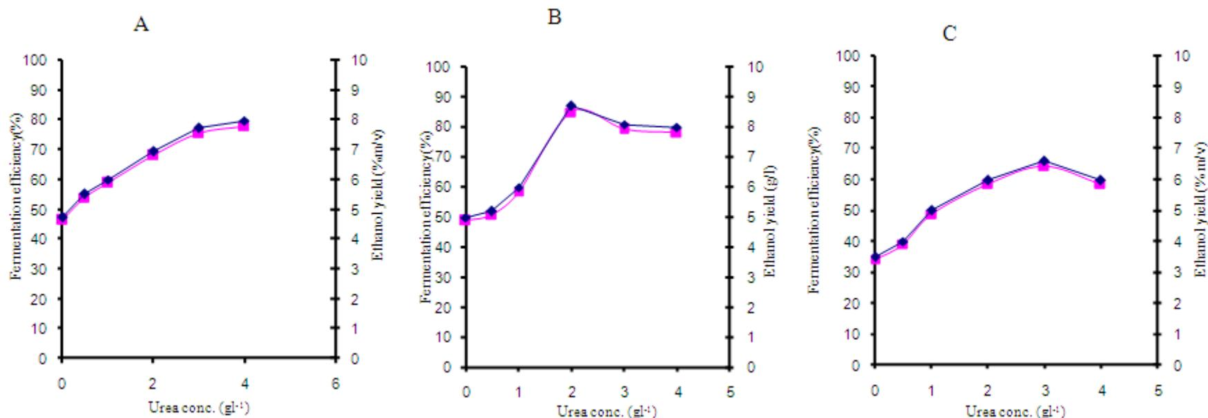
**Figure 1.** (A-C) Graphical representation of ethanol yield ( $\text{g l}^{-1}$ ) ( $\blacklozenge$ ) and % fermentation efficiency ( $\blacksquare$ ) on molasses medium supplemented with urea concentrations between 0-4  $\text{g l}^{-1}$  at 30°C (A), 35°C (B) and 40°C (C).
