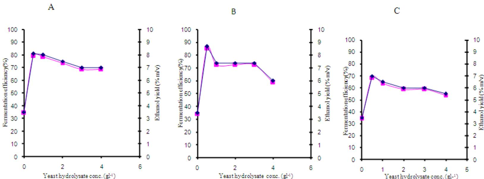
**Figure 2.** (A-C) Graphical representation of ethanol yield ( $\text{gl}^{-1}$ ) ( $\blacklozenge$ ) and fermentation efficiency ( $\blacksquare$ ) on molasses medium supplemented with yeast hydrolysate concentrations between 0 to 4  $\text{gl}^{-1}$  at 30°C (A), 35°C (B) and 40°C (C).
