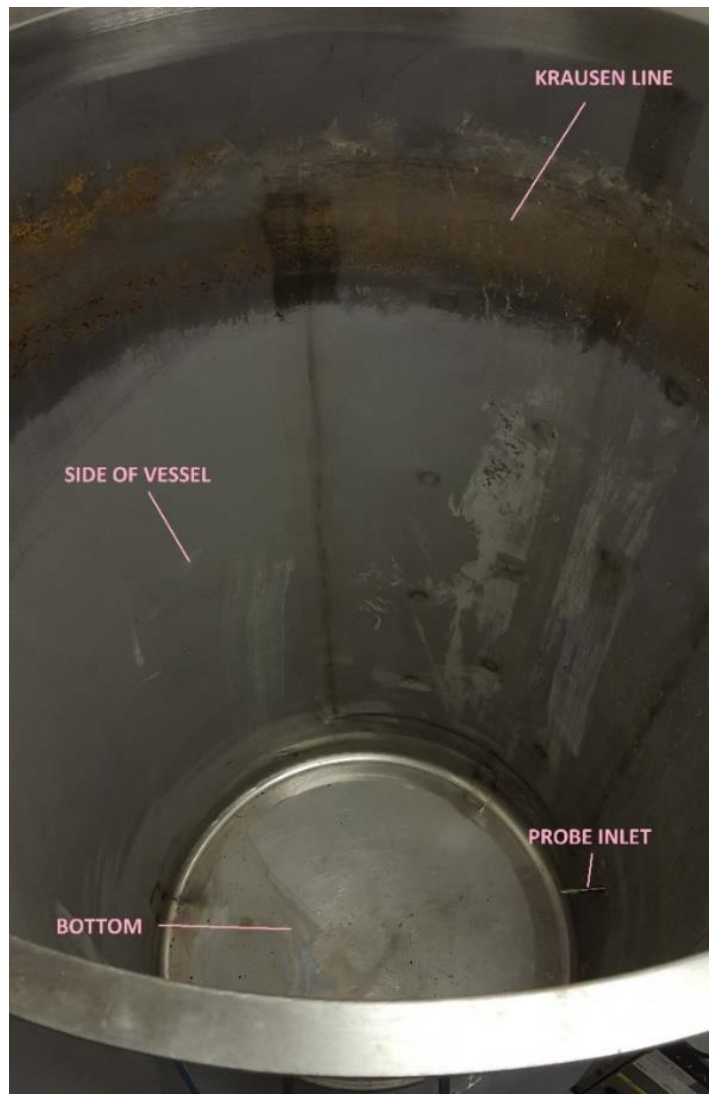
Figure 2. Inside of a typical cylindrical microbrewery fermenter after fermentation, with a specific highlight on the Krausen, Interior side wall and an example 'Other' area (Probe Inlet).
